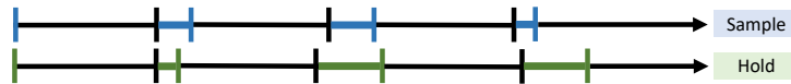
FIGURE 34 Example 22: Timing diagram for relative clock jitter with asynchronous A/D and D/A devices. The interval between the blue and green vertical bars and the black vertical bars indicates the nominal relative clock intervals.
