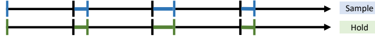
FIGURE 32 Example 21: Timing diagram for relative clock jitter with synchronous A/D and D/A devices. The interval between the blue and green vertical bars and the black vertical bars indicates the nominal relative clock intervals.
