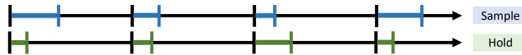
FIGURE 30 Example 20: Timing diagram for absolute clock jitter with asynchronous A/D and D/A devices. The black vertical bars indicate the nominal absolute clock intervals.
