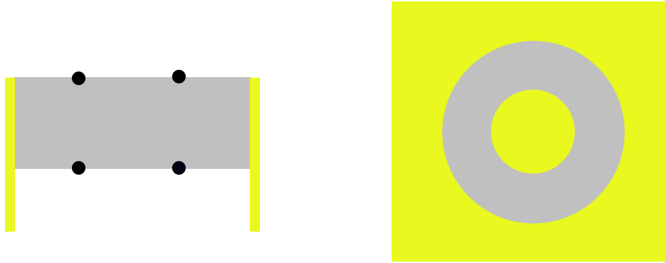
Figure 1.3: Electrical Transport Geometries. Left: Hall bar geometry. Current is fed in through the gold contacts on the left and right, and the voltage measured at the black points. The upper and lower boundaries are insulating. Right: Corbino disk. The voltage is measured between the inner and outer contacts (gold). Since there is no insulating boundary, the Hall conductivity is suppressed.
