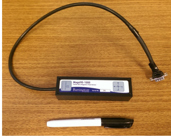
Figure 4.6: A Bartington Mag690-1000 fluxgate used in the experiment. Sharpie for scale.
