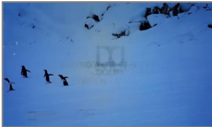
Figure 5-1. An example of burn-in in OLED devices.
