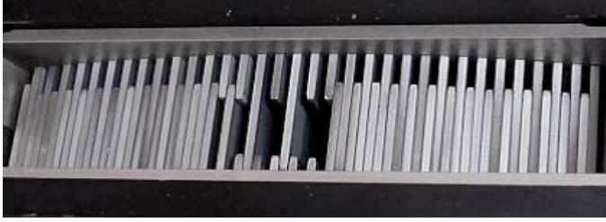
(a) Binary Multi-Leaf Collimator (tomotherapy); each leaf is either completely open or closed.
