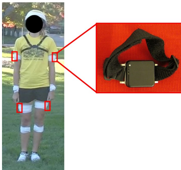
Figure 5.1: Participant with four IMUs attached to upper arms and thighs (red boxes) and a callout of an IMU node on the right.
