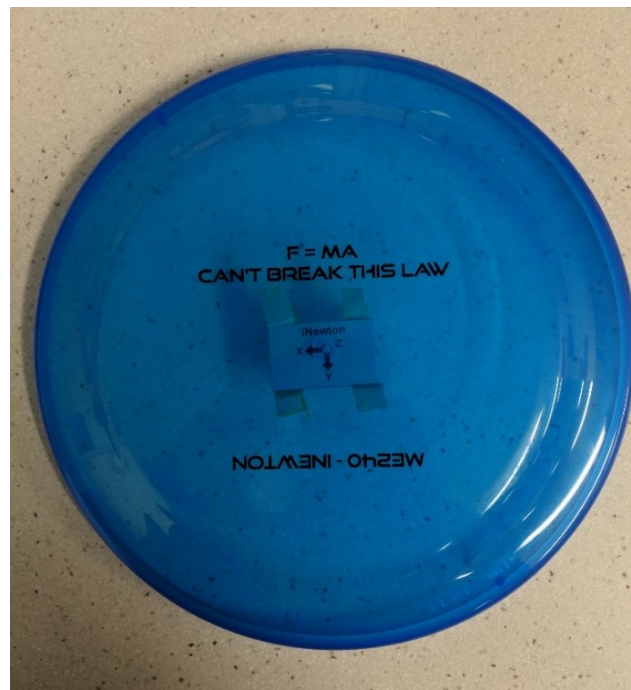
Figure 8.7: An example configuration for the iNewton sensor attached to the Frisbee (Prescribed Experiment #2).
