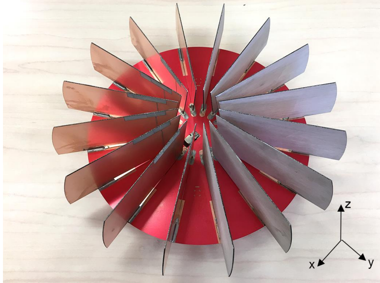
Figure 3.15. Fabricated CP antenna, the ground plane includes red solder mask [16].
