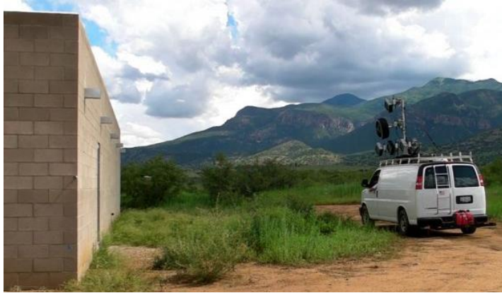
Figure 1.1. Large antenna array mounted on a vehicle for through-the-wall imaging from outside of the building ( www.eurekaerospace.com ).
