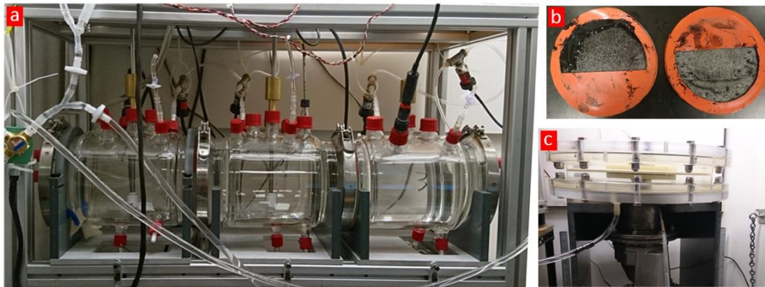
Figure 4.5: The BfE-AnMBR treats wastewater by sending it through three compartments in series (a) separated by meshes that serve for biofilm attachment (b) and filtering it using a rotating disk membrane (c). Picture (b) shows the mesh-biofilms.
