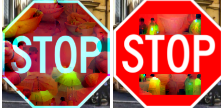
Figure 4.4: Output of the extended RPP algorithm to attack YOLO v2 using poster and sticker attacks.
