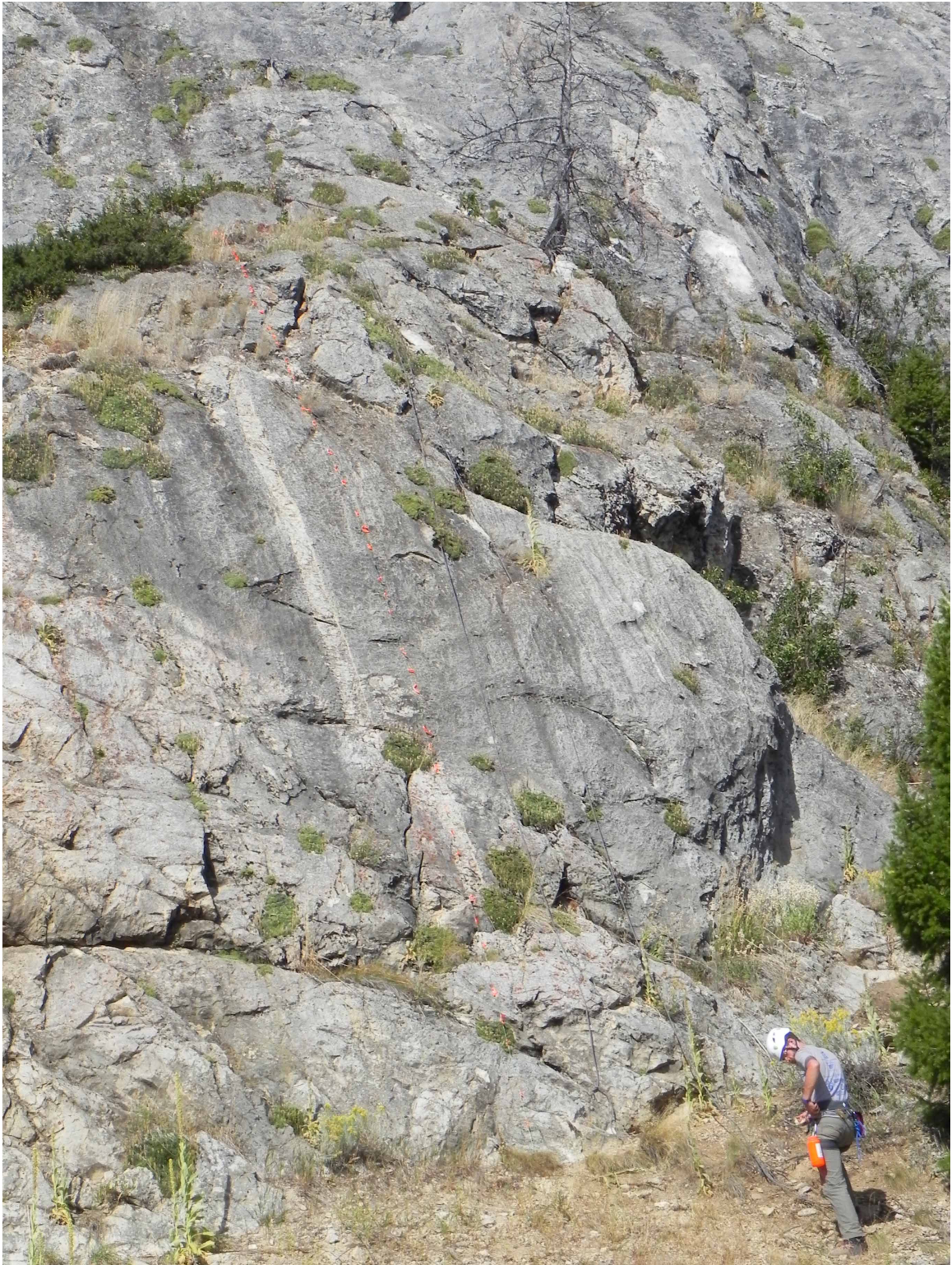
Figure B.1: Full-size photograph of the Hebgen fault exposure showing string line and orange flagging to locate Schmidt hammer sample locations every 0.25 m.
