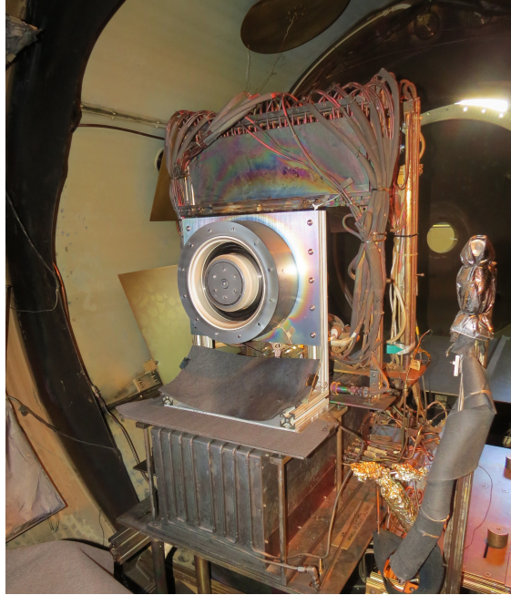
Figure A.2: The H9 SN03 installed in the Owen's Chamber at the Jet Propulsion Laboratory for thrust measurement testing.
