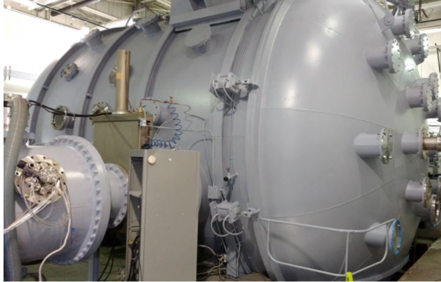
Figure 4.7: The Large Vacuum Test Facility at the University of Michigan.
