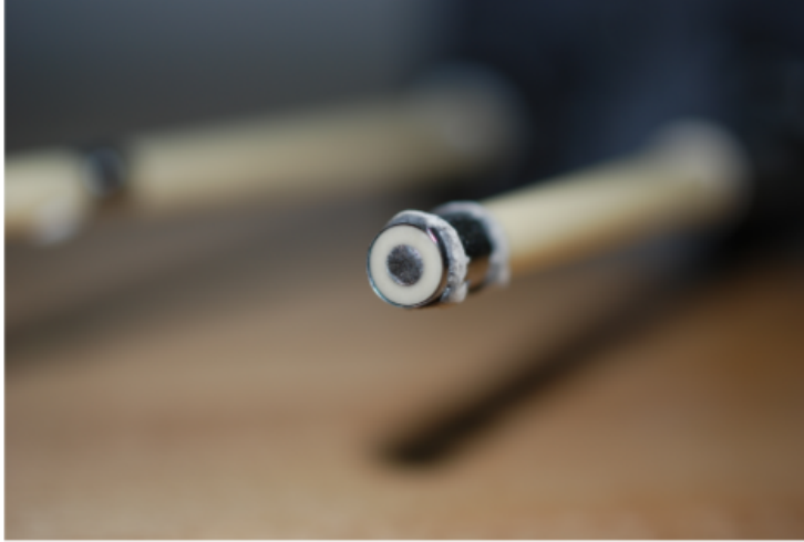
Figure 4.10: Near-field Faraday probe featuring a tungsten collector plate and guard ring.
