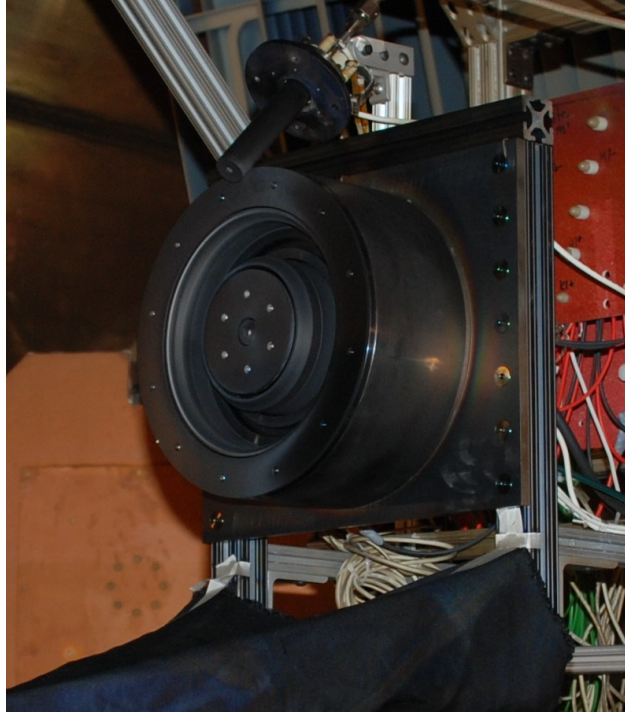
Figure A.8: The H9 after approximately 100 hours of firing at the University of Michigan. Build up of carbon along the entirety of the discharge chamber walls is a qualitative indication of achieving a magnetic shielding topology.
