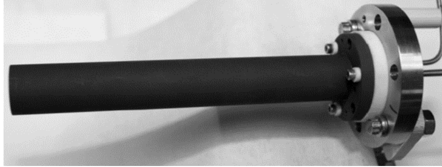
Figure 4.5: One of the 20-A class cathodes used during these investigations. This cathode has the traditional sheath heater and was used for the X2 and some H9 experiments.
