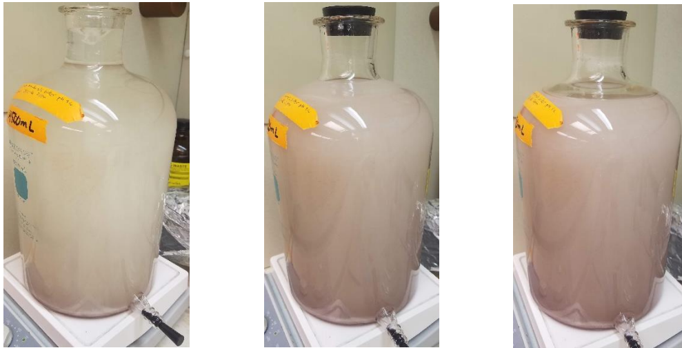
Figure B-3 Lead carbonate batch reaction over the course of one hour. Image 1 was taken immediately upon the addition of lead carbonate. Images 2 and 3 are taken after late batch reaction samples.
