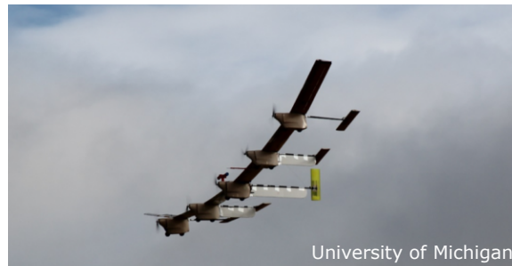
Figure 1.3: 6-m X-HALE experimental testbed during flight.
