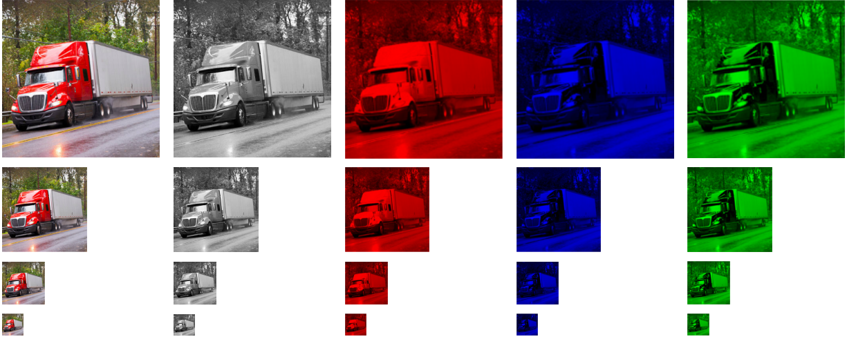
Figure 1.2: Examples of the variations in input representations created to increase the design space of TAHOMA’s cascades. Tiny images with a single color channel lead to much faster classifiers, due to a much small number of input parameters. These tiny inputs may carry sufficient information to successfully answer some queries.
