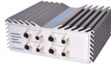
Figure 3.3: Speedgoat® controller and its configuration.
