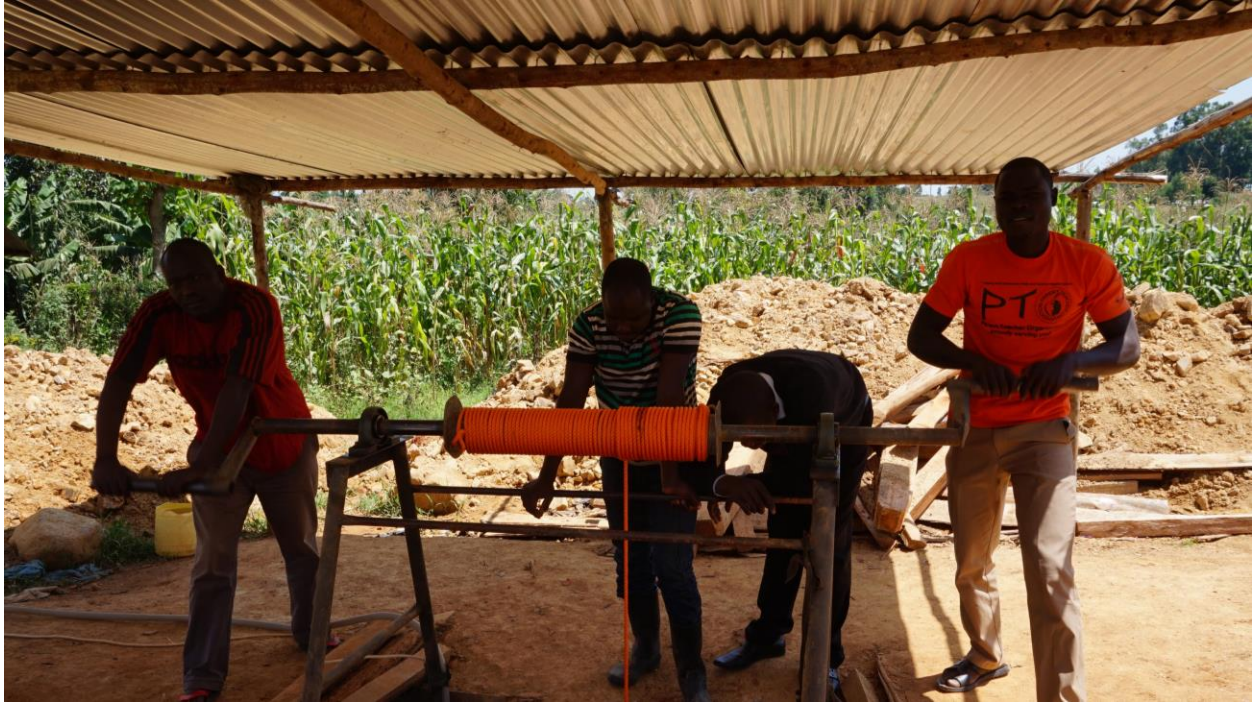
Figure 6: Male miners working a pulley to lower a miner into the mineshaft, Source: Author.
