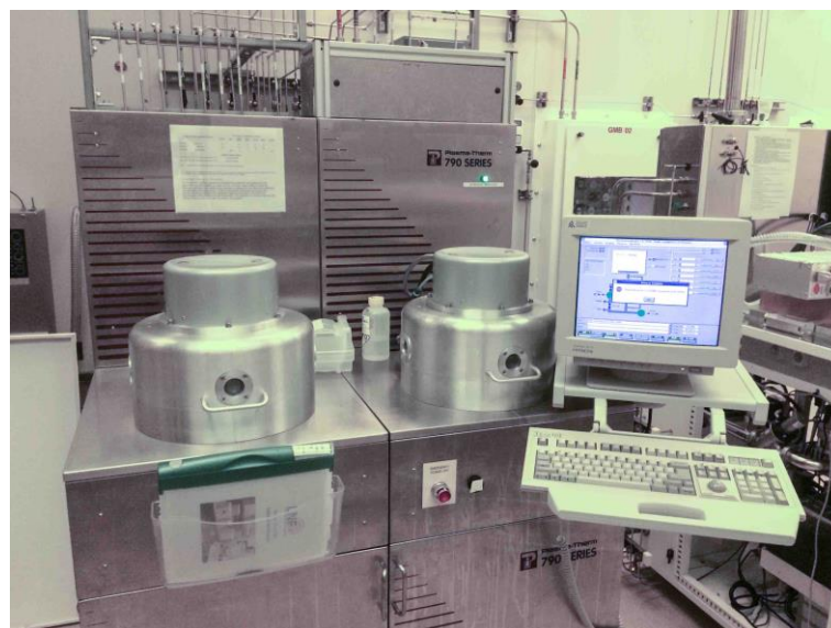
Figure 1.9 PECVD Plasmatherm 790 for a-Si deposition, which is used for the a-Si active layers in the devices we worked on.
