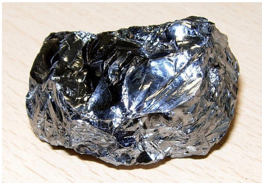
Figure 1.1 Silicon ingot after preliminary purifications. (Reproduced from [1]).
