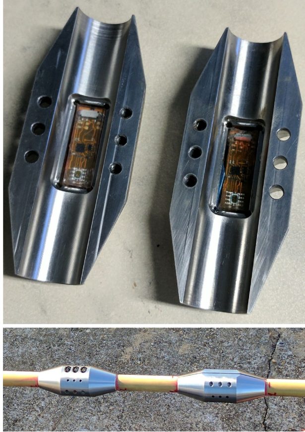
Fig. 3. 7: The ELM systems are laid flat inside metal clamps, which are then tightened around a JONC rod and lowered into the well.
