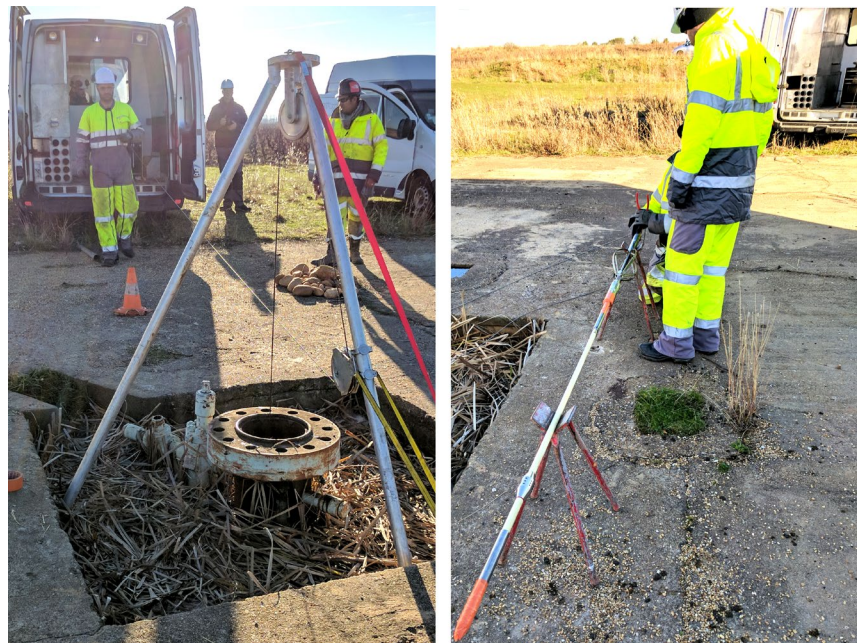
Fig. 3. 6: Field testing. A wireline runs from a winch situated in a truck (left), which lowers the microsystems into the well. The systems are attached to a JONC rod (right) using metal clamps. A macroscale wireline monitor is also connected to the rod for reference.
