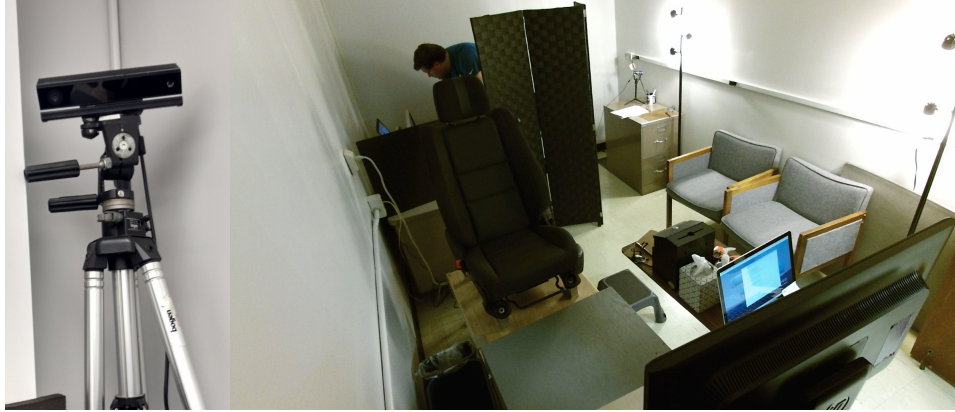
Figure 3. Kinect (left) and Kinect field of view showing laboratory setup
