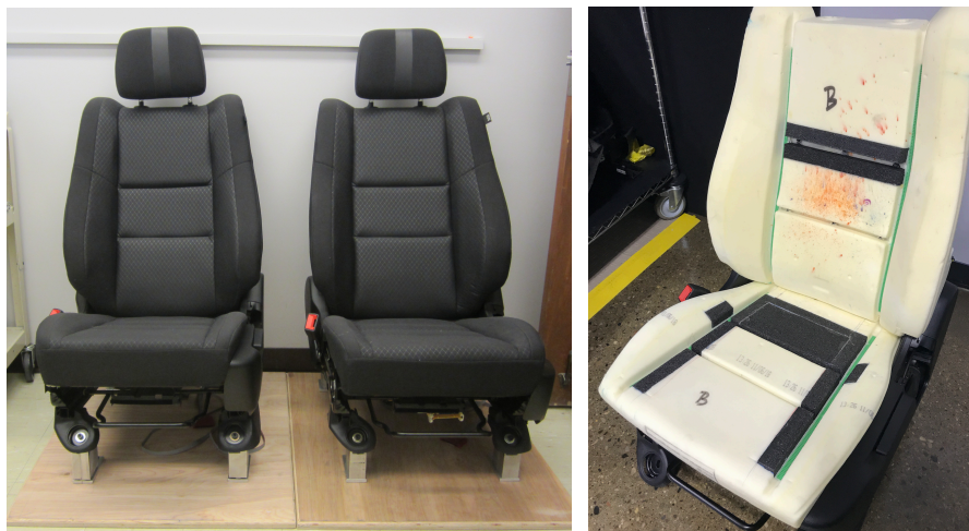
Figure 1. The standard Seat A and modified softness Seat B from left to right; photo of Seat B showing modified foam areas (dark).
