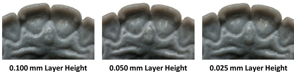
Figure 2. Palatal views of the incisors of 3D printed models showing increasing surface smoothness with decreasing layer heights of 0.100 mm, 0.050 mm, and 0.025 mm.
