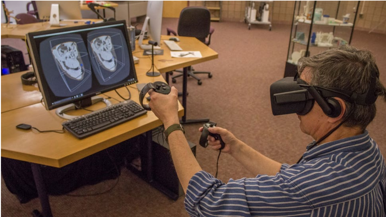
Figure 1. Jaw simulation using Virtual Reality Patient with Oculus Rift head mounted device and touch controllers.
