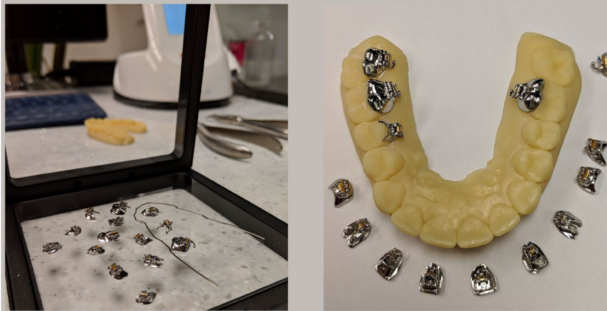
Figure 10: The complete set of Chrome Cobalt custom printed brackets are shown in this figure along with the custom wire hand bent from a 2D 1:1 printed wire card.
