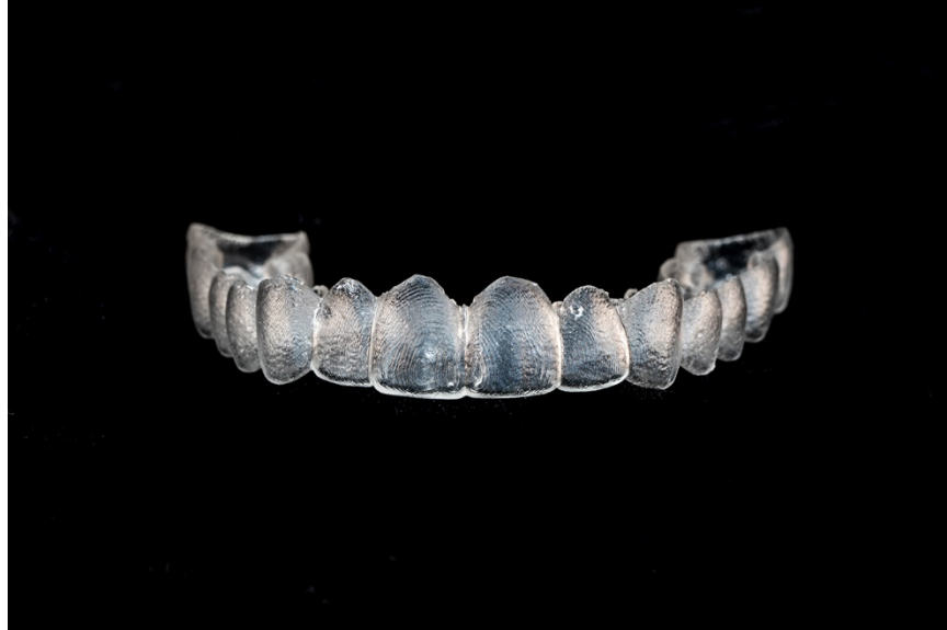
Figure 6. Photograph of a clear aligner fabricated directly via 3D printing in a resin cleared for intraoral use for production of occlusal splints. The aligner was designed digitally to fit a scan of a typodont and is shown after removal of the supporting structures.
