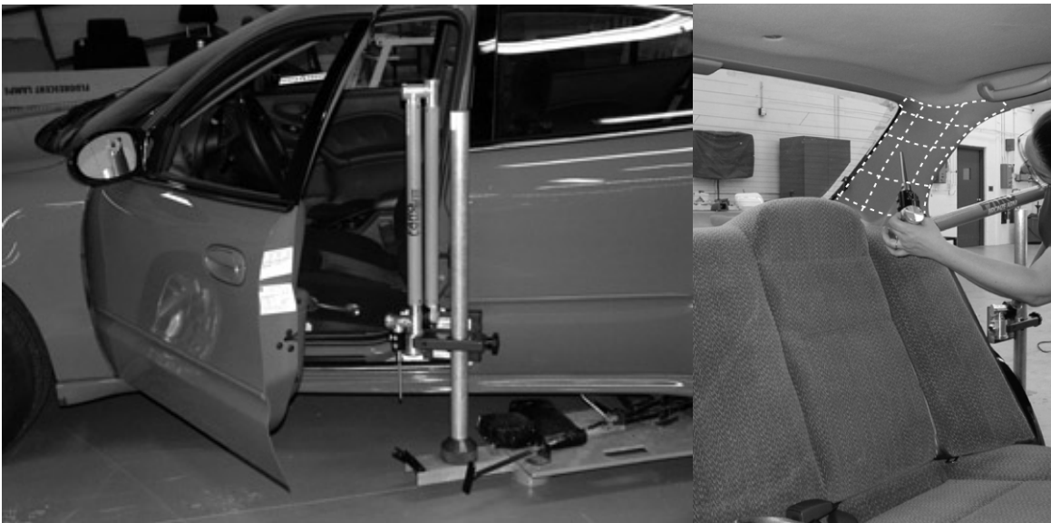
Figure 1: FARO arm shown mounted to a vehicle (left) and being used to digitize the shape of vehicle pillar (right) in a grid pattern.
