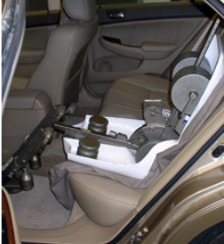
Figure 2: Measuring the location of the rear seat H-point
