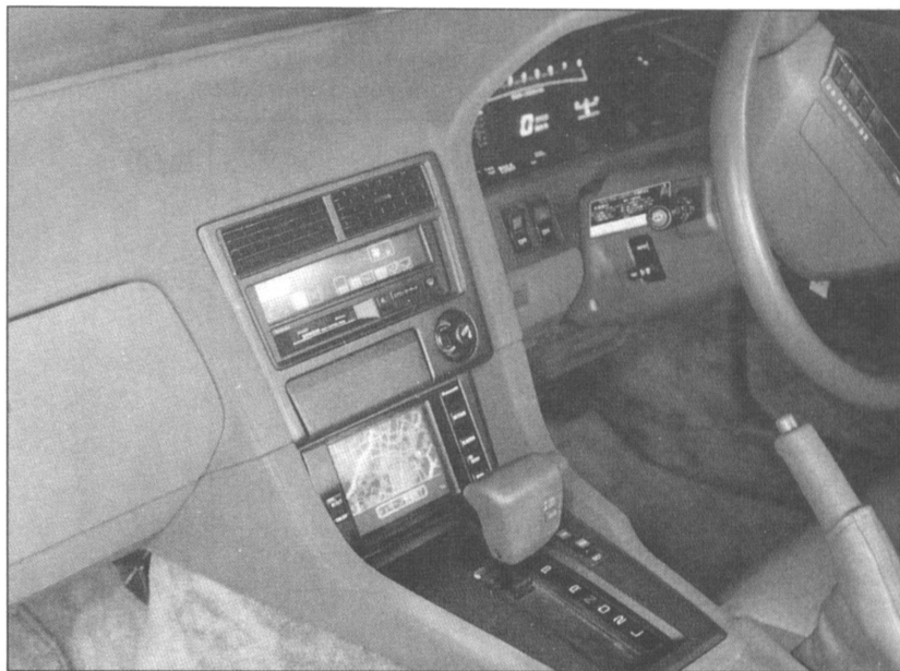
Figure 8.5 Photo of navigator screen installed in RACS experiment vehicle (with illustrations, from top to bottom, of screen display for traveler service information, guidance, and vehicle location on the map).
