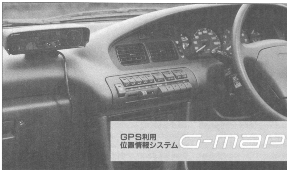
Figure 8.11 G-Map Display unit, at left, constituting an aftermarket GPS-based navigator built by Aisin Seiki and marketed through Toyota dealers.
