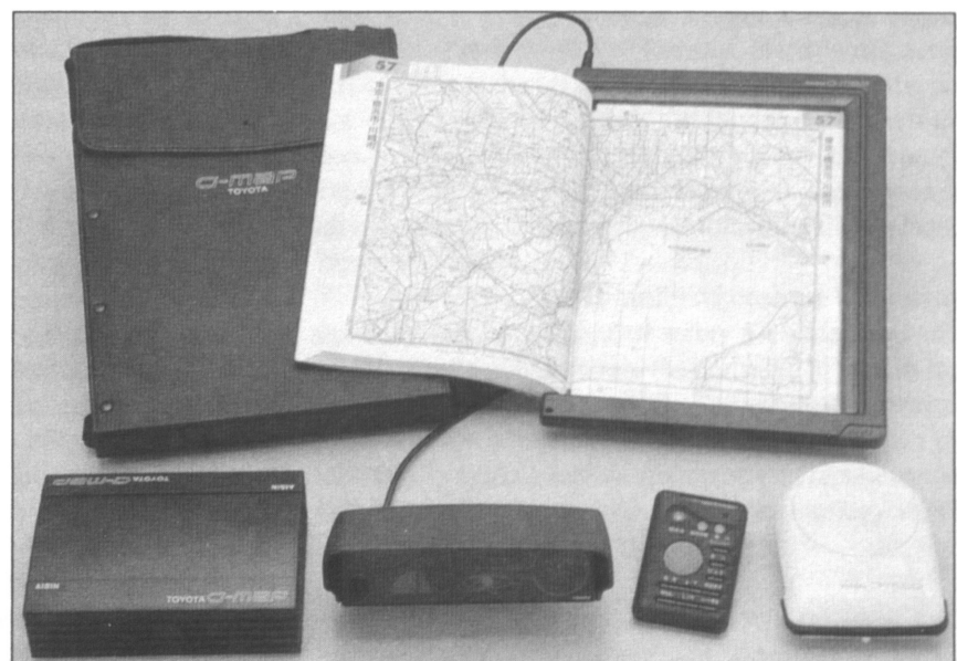
Figure 8.12 Package of G-Map components showing, upper right, a Standard Road Map inserted within the LED Digitizing Frame, for entering reference points comprising a desired route.
