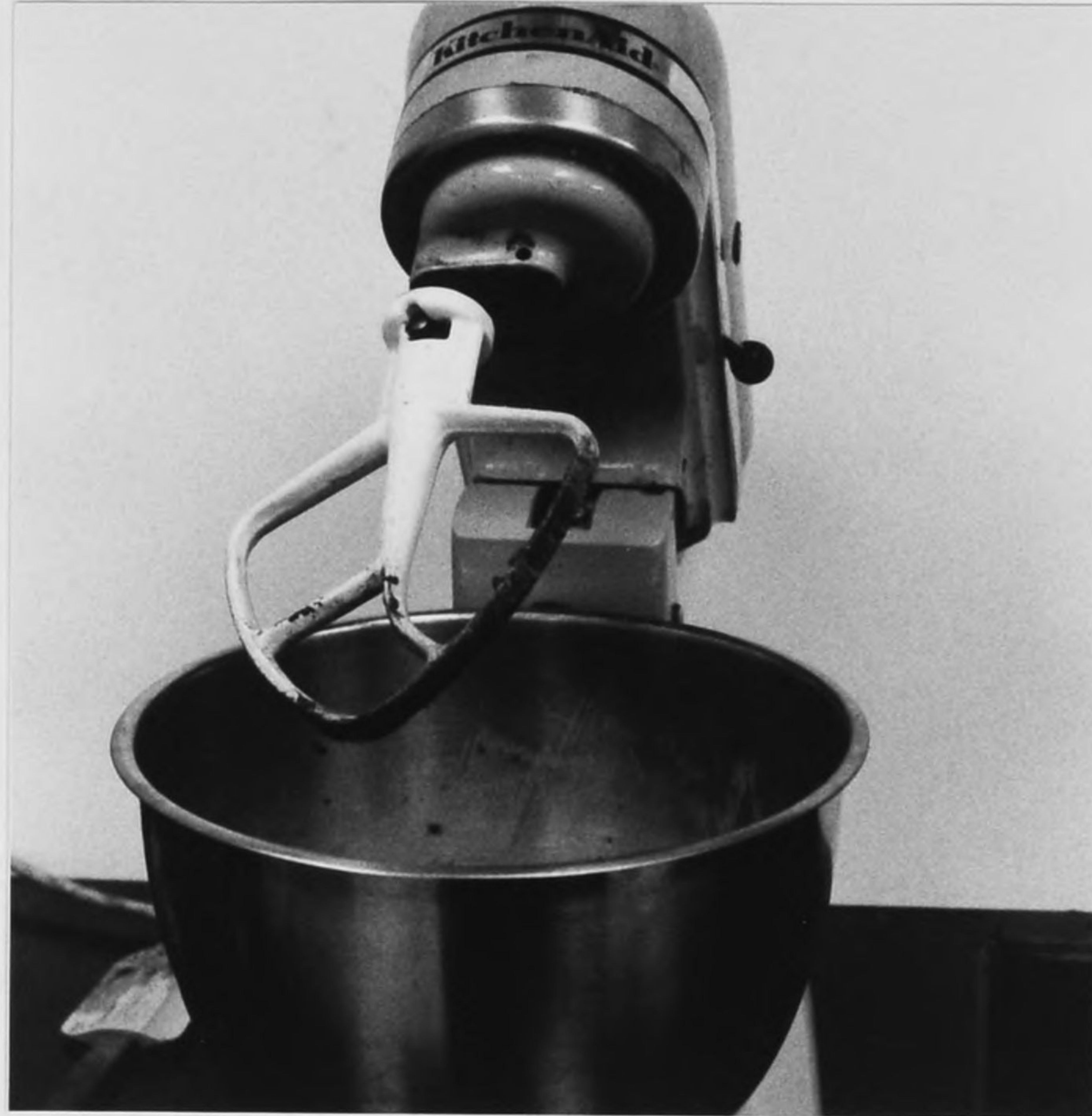
Figure 8. Heavy duty, variable speed food mixer used to mix fly ash, cement, and water in laboratory.
