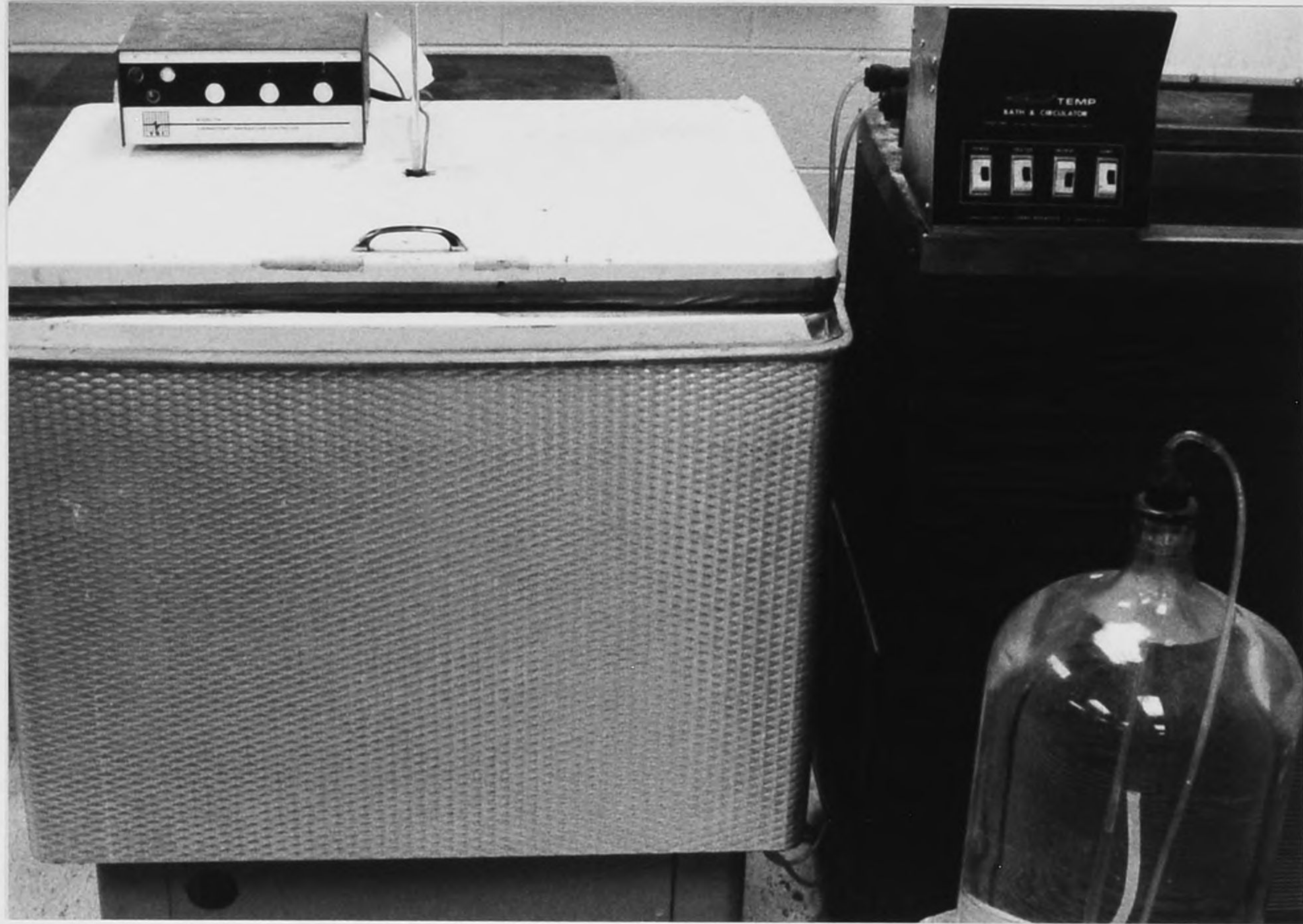
Figure 14. View of frost cabinet (to left), water temperature controller (atop cabinet), and water circulator (on right).
