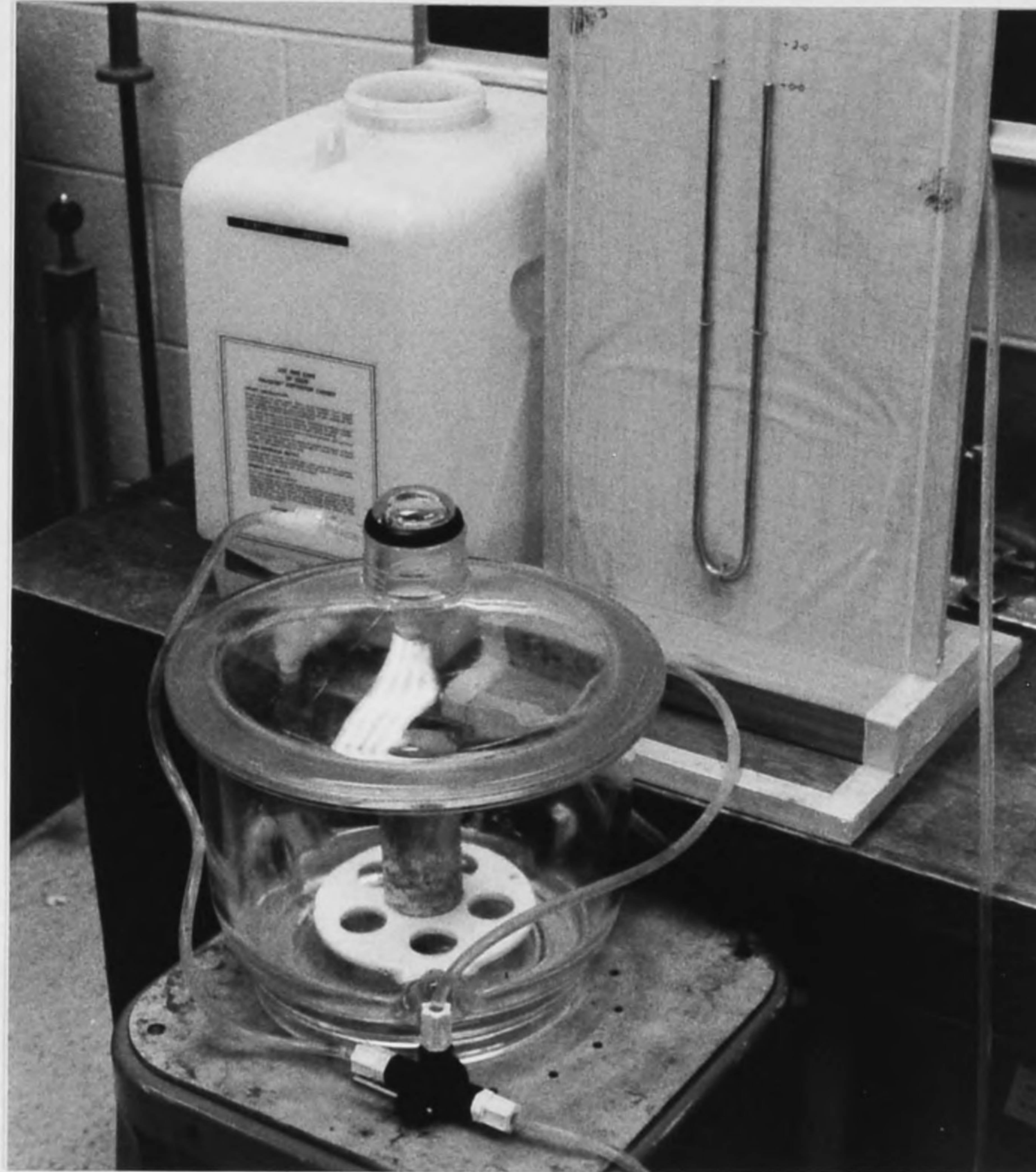
Figure 13. Vacuum saturation apparatus used for evacuating samples and inundating them in distilled water
