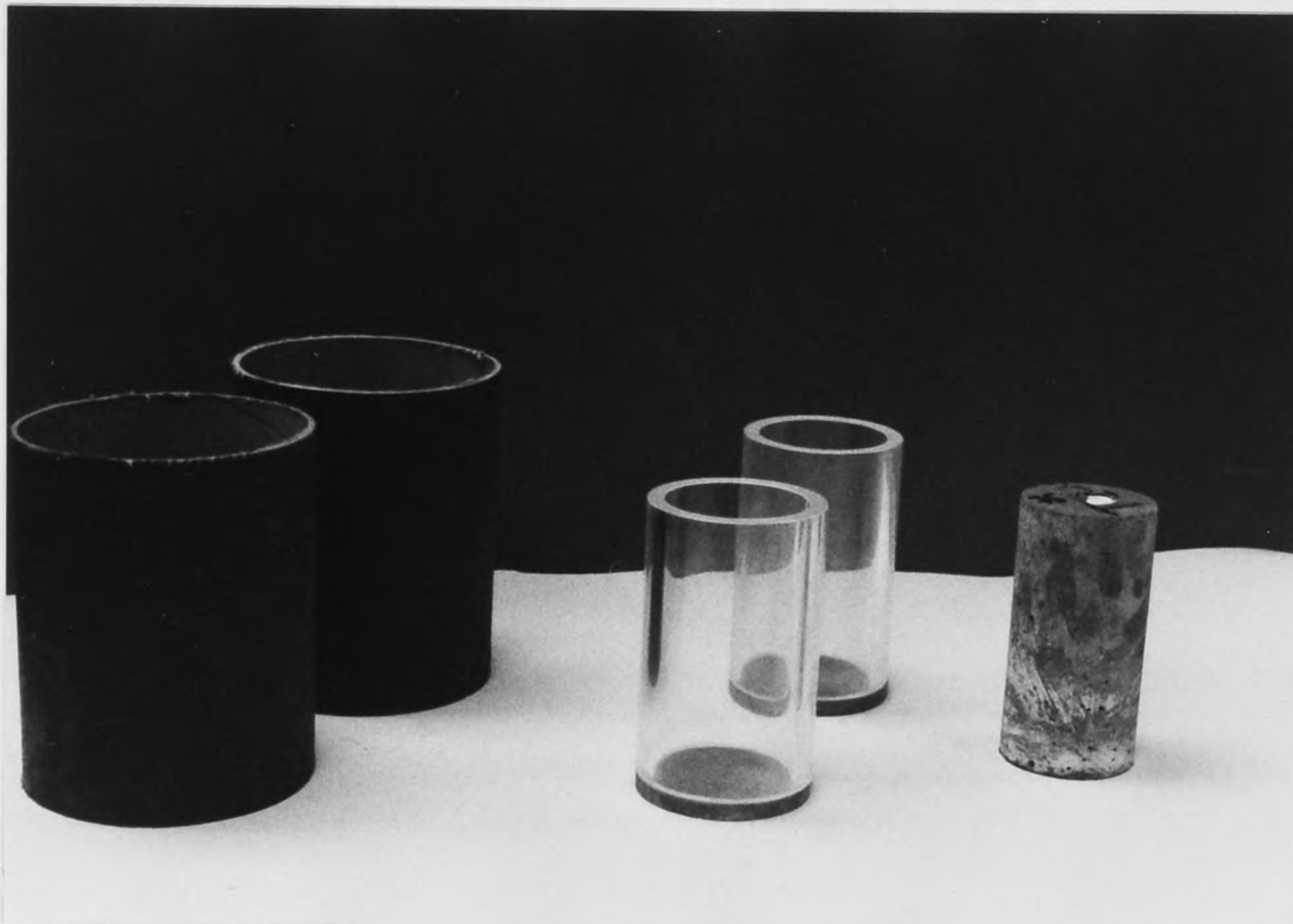
Figure 10. Casting molds--4-inch diameter cardboard tubes and 2-inch diameter acrylic molds and porous stone used to cast fly ash/cement mixes.
