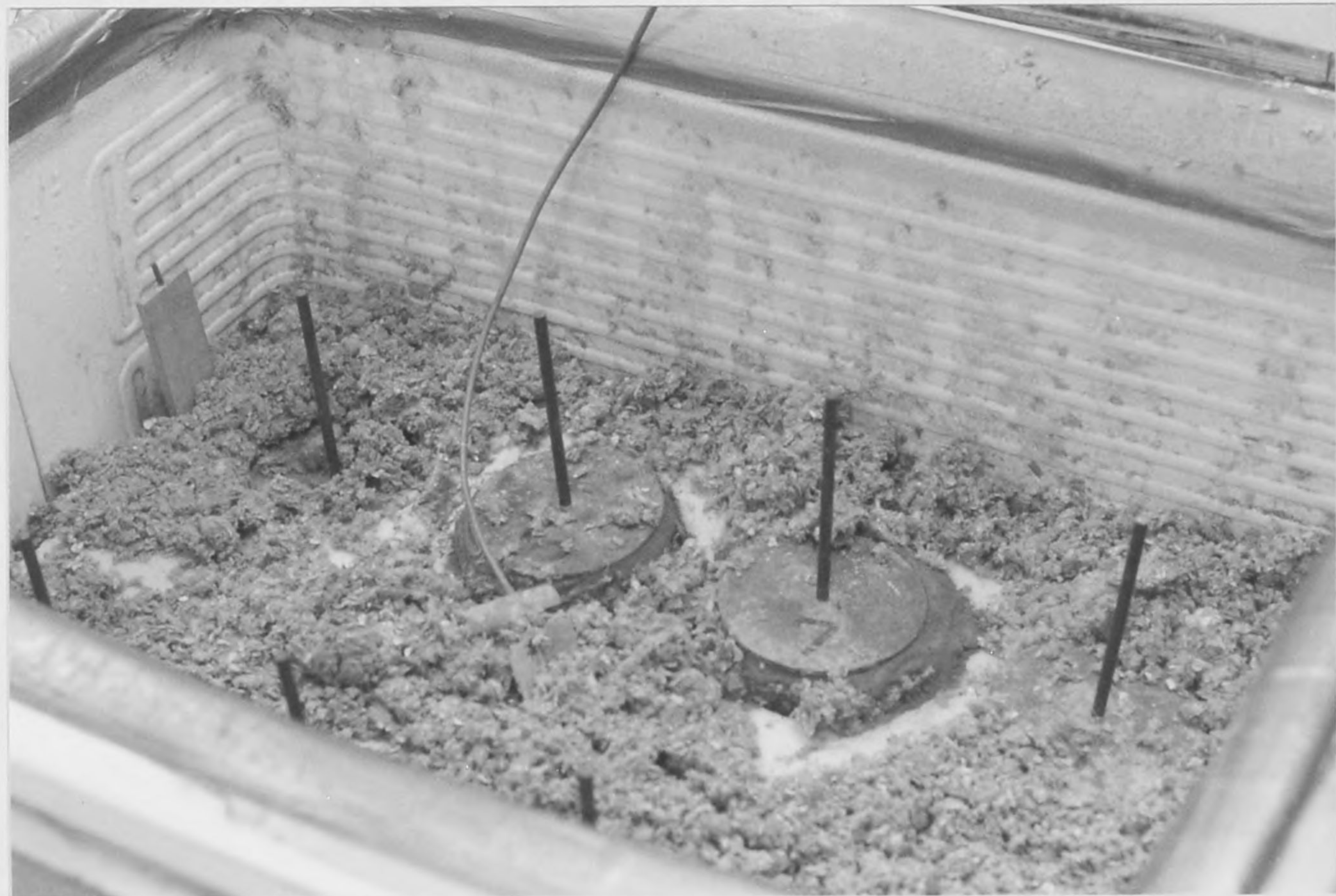
Figure 15. Inside view of frost cabinet showing sample tops protruding above insulation and heave reference bars.
