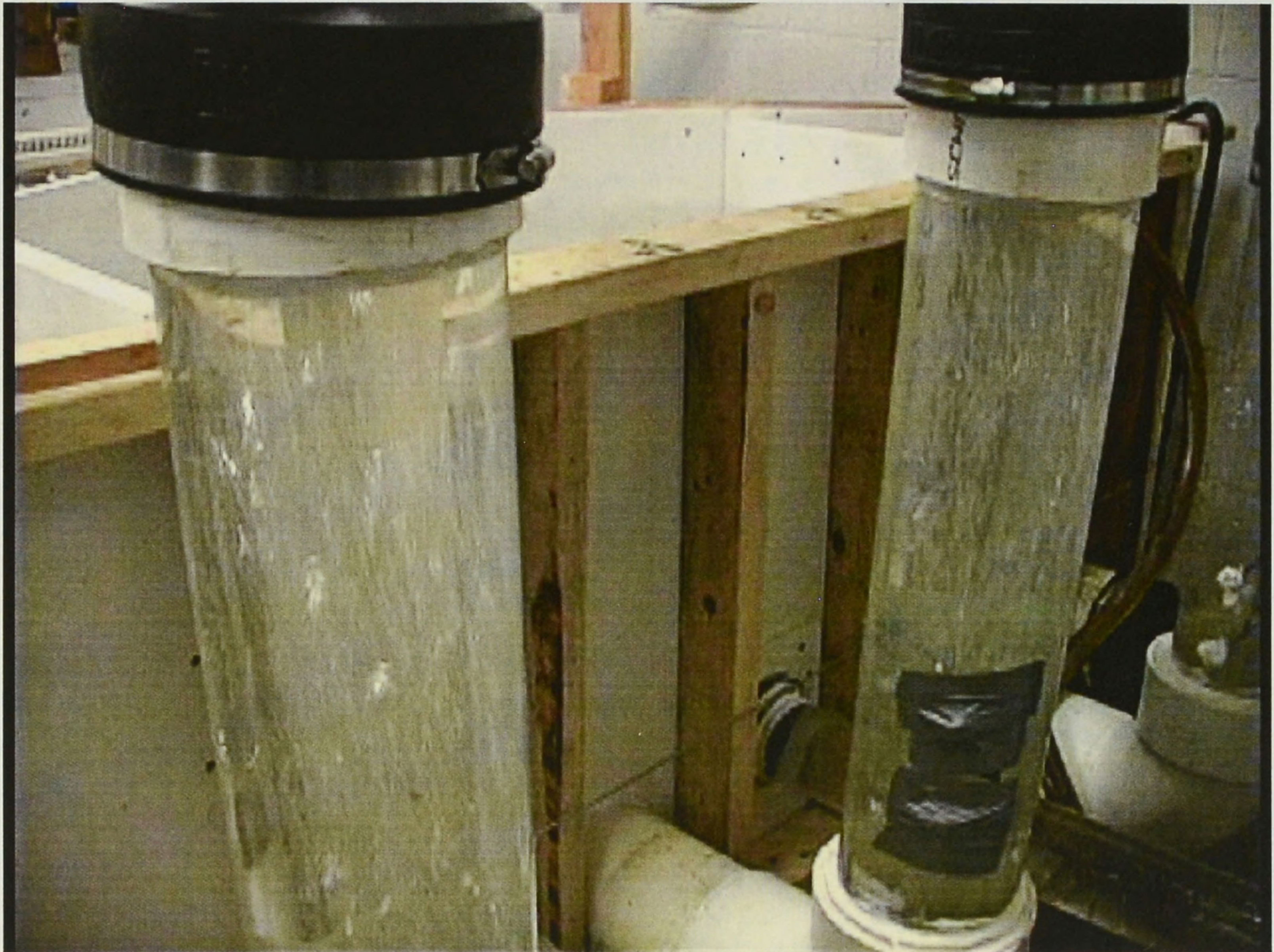
Figure 9. Air Entrainment into Pumps 5 and 6, for a low wet well level.
