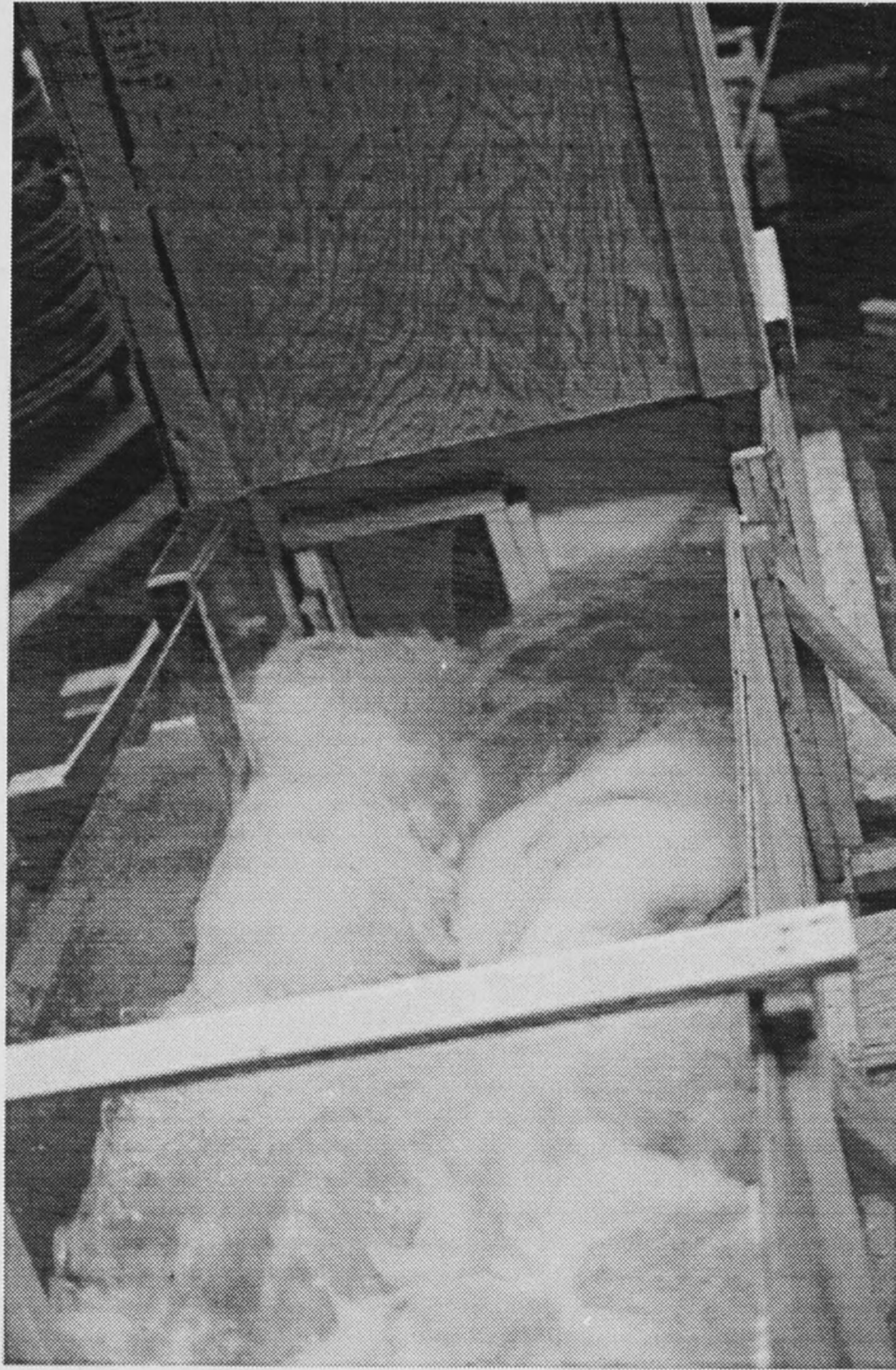
Figure 6d: Top view of testing results of modified Revision 2 design at 243 cfs.
