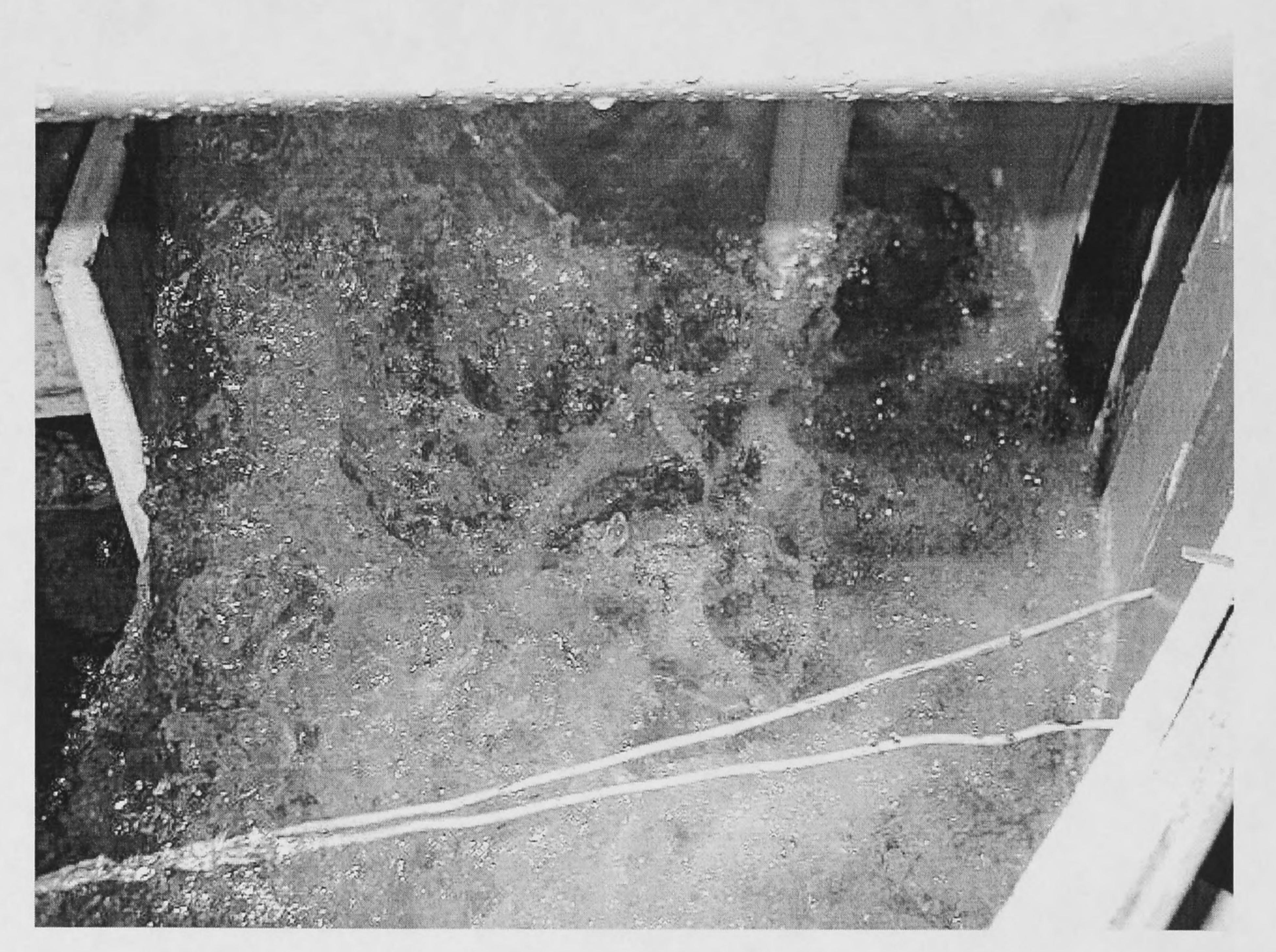
Figure 7. Nature of Flow in Inlet Chamber with Six Pumps in Operation at the High Water Level (Start the sixth pump). This image was taken after the design modifications were made.
