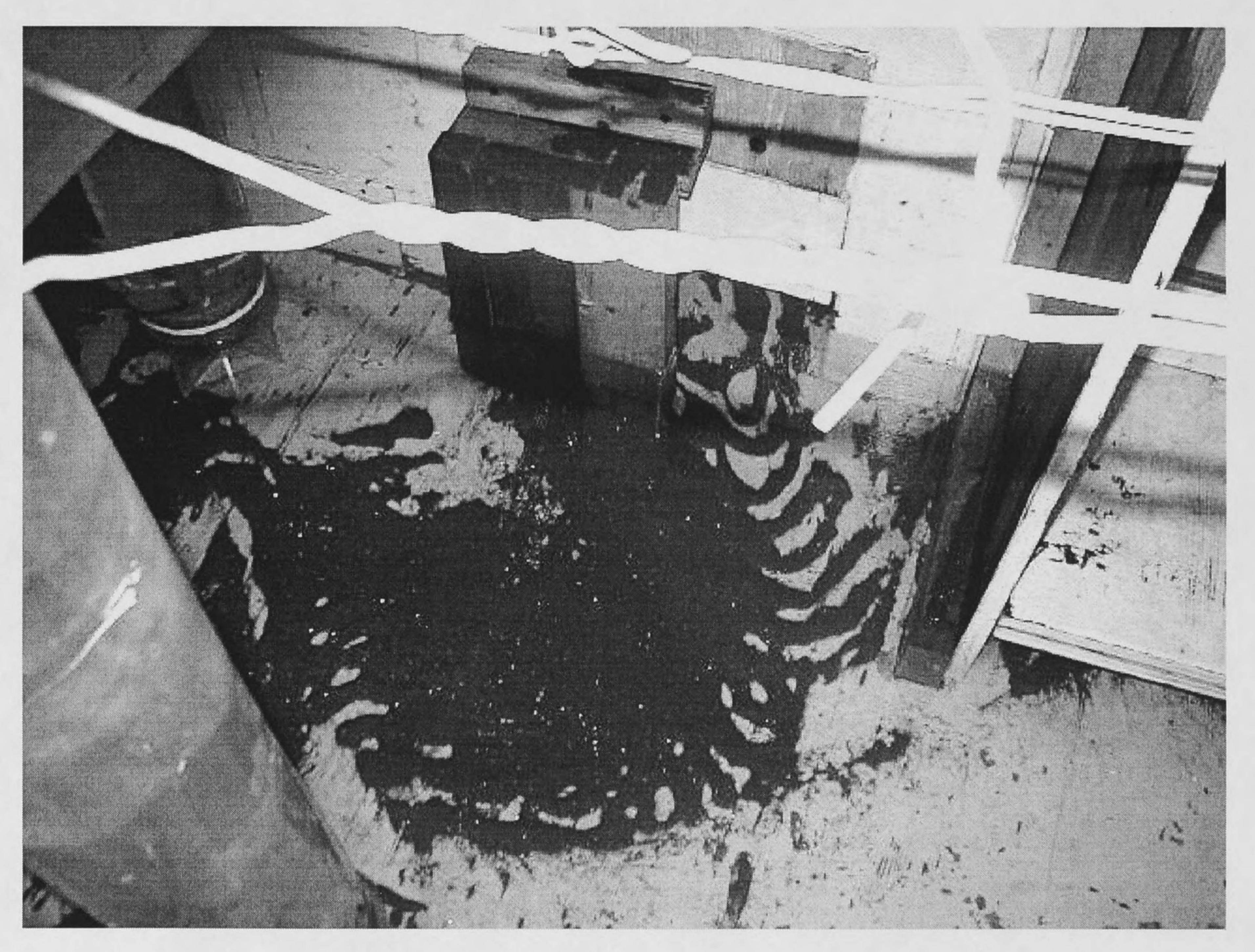
Figure 15. Sedimentation Patterns in Front of Intakes 2 and 3.
