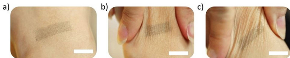
Figure S1. Optical images of transfer-printed PEDOT:PSS thin films, with a thickness of 100 nm, from glass substrates onto skin: a) after transferring; b) under mechanical compression; and c) under mechanical distortion. The scale bar is 1 cm.
