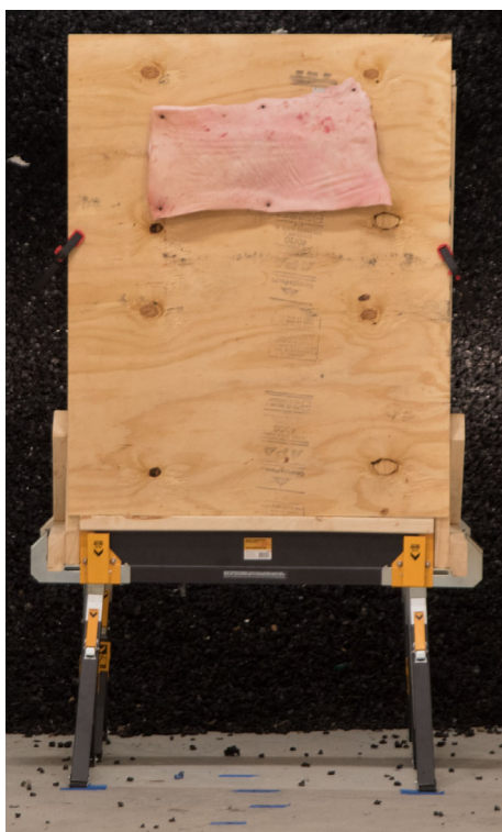
FIG. 1—Target stand supporting abdominal wall segment. [Color figure can be viewed at wileyonlinelibrary.com ]
