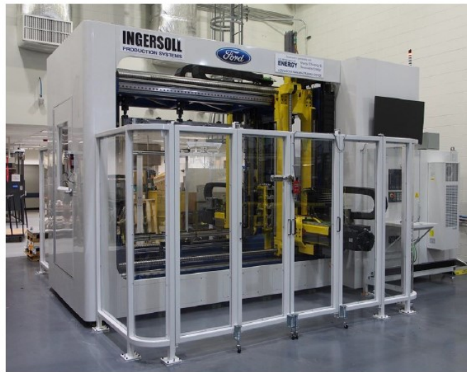
Figure 1: ISF process and machine
