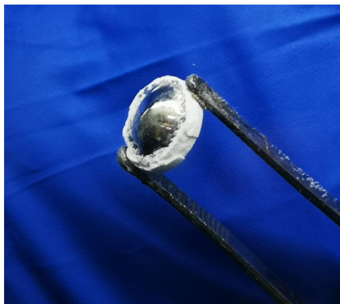
Fig. S12 Digital photos of the melted Li metal on top of the pure \text{Li}_2\text{CO}_3 pellets after rub-coating molten Li.
