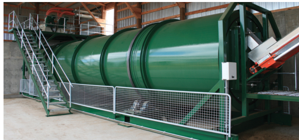
Figure 5. The “Ecoponics” In-Vessel compost system processes food waste in a contained system to reduce odors and pest concerns.
