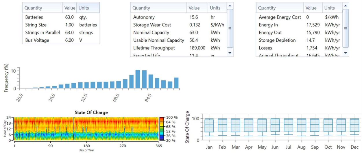
Figure 53. Phase III grid-isolated biomass battery summary.
