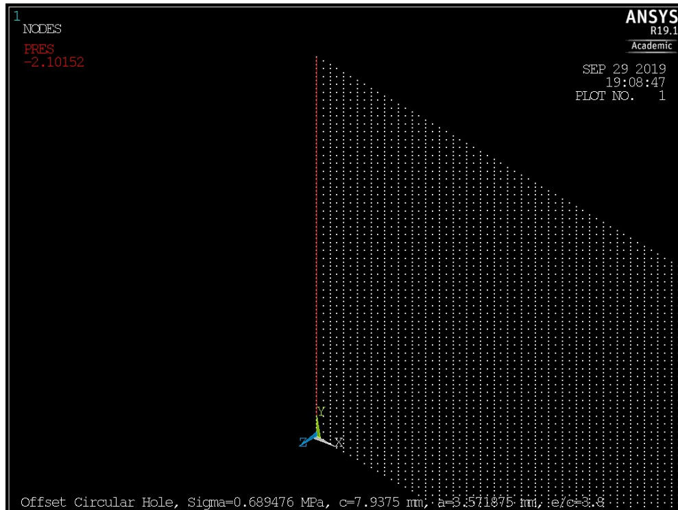
Figure 3.16: Applied negative uniform linear load at x = 0 , for the SHELL281 laminate.
