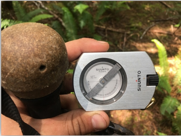
Figure 40 Clinometer used for measuring slope throughout these proposed routes during the trail design process (Pritchard 2018)
