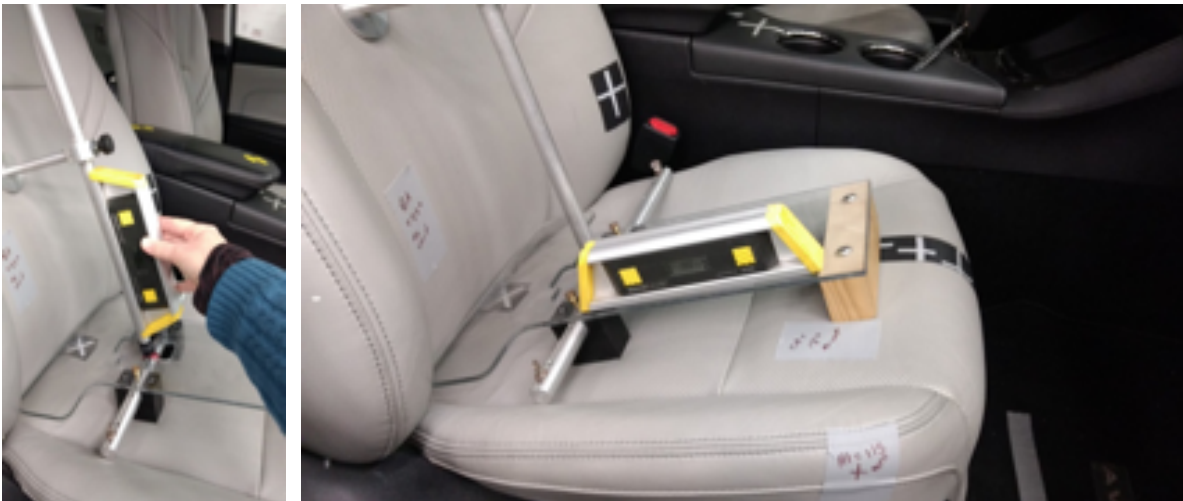
Figure 6. Investigator measuring seat back angle (left) and seat pan angle (right) using tool (Huang and Reed 2006; Klinich et al. 2013) and inclinometer.
