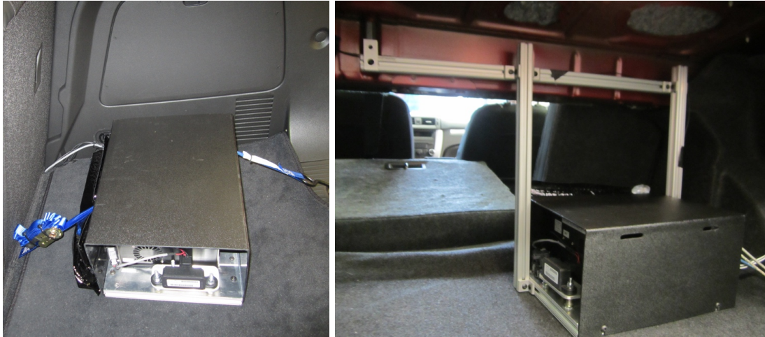
Figure 2. Data acquisition system (DAS) in the trunk of a vehicles
