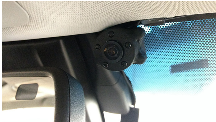
Figure 1. Cabin view camera with IR illuminators mounted in vehicle
