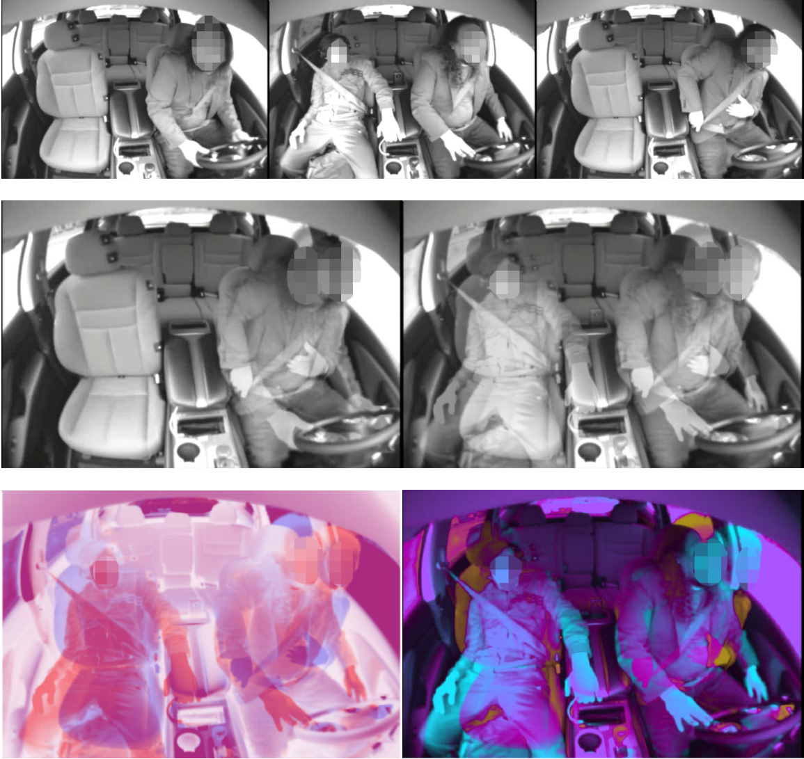
Figure 14. Video frames from start, middle and end (top row, left to right) of a trip with seat movement and transparency of the start frame overlaid onto end frame and middle frame onto end frame (middle, left to right). The bottom row shows overlaid images colorized and with the differences highlighted.
