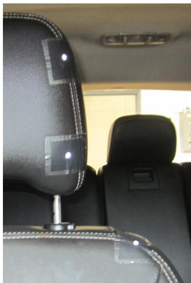
Figure 7. Retroreflective markers on a vehicle seat
