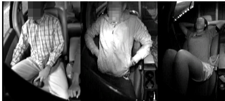
Figure 41. Upper back not touching seat back in a standard posture (left), touching seatback in a slouched posture (center), and touching the seatback in a reclined posture (right)
