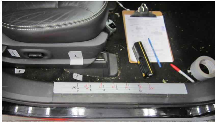
Figure 9. Tape on vehicle seat and frame to mark arrival position in vehicle with adjustable seat height
