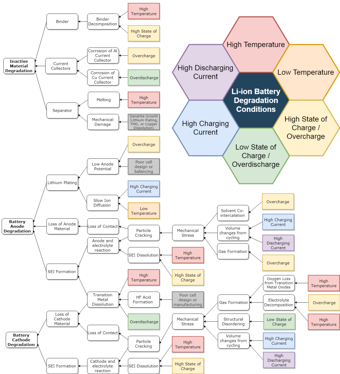
Figure 2. Degradation mechanisms in Li-ion batteries.
