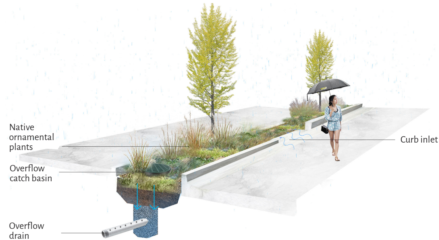
▲ Bioswales or rain gardens adjoining impervious surfaces like streets or parking lots can help capture and infiltrate stormwater runoff.
