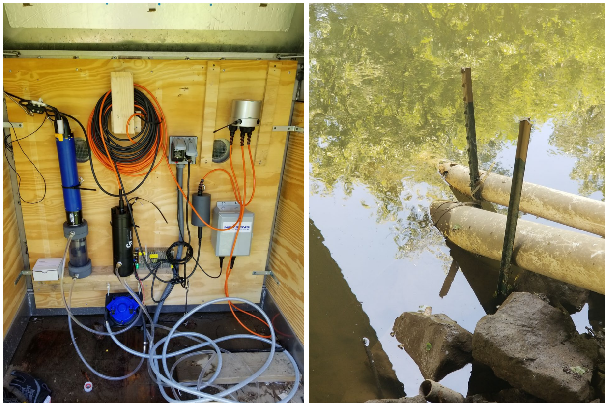
Figure 3-1: Comparison of pump and flow-through cell (left) versus in-situ deployment (right) monitoring configurations. Pump and flow-through cell configuration includes a peristaltic pump, bringing surface water in series through the YSI EXO 2 and Turner Designs C3™ water quality sondes, and outflow back into the stream, as well as power and telemetry devices. The in-situ deployment includes both water quality sondes deployed directly in-stream and protective PVC housing with flow openings (power and telemetry devices are not shown).
