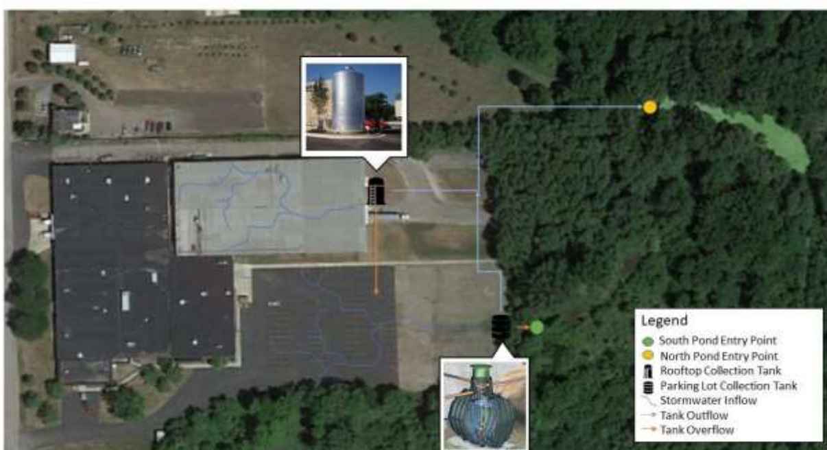
Figure 24. Diagram of proposed rerouting of stormwater off the Kiwanis Club warehouse and parking lot into the North and South Ponds. Aerial image from Google Earth. Pop-up images from RainHarvest.com. Not to scale.
