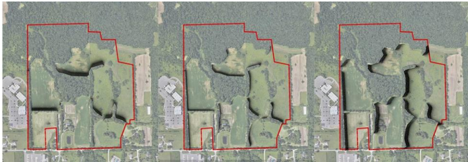
Figure 12: Shade condition in January- 9 AM, 12 AM, and 4 PM
