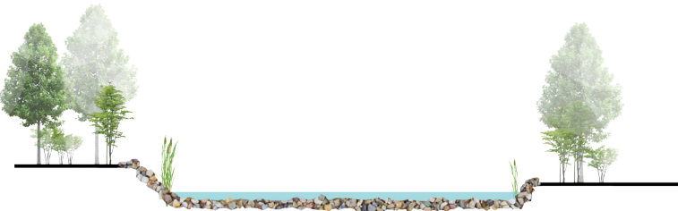
Figure-71. After- taking into account increased water flow to the site, there is consistent water retained on site and visual interest is added with stonework and vegetation.
