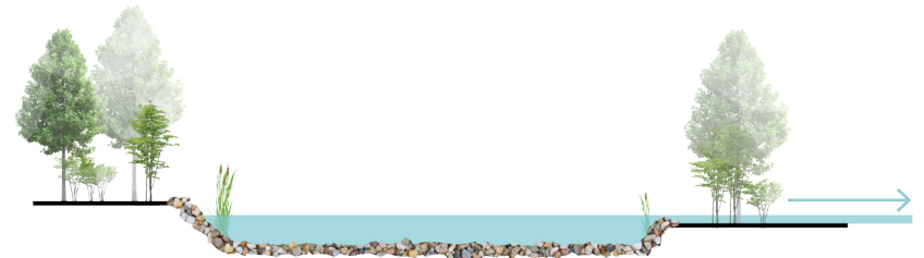
Figure-73. After- In the event of highwater conditions, water can slowly flow to the wetland.
