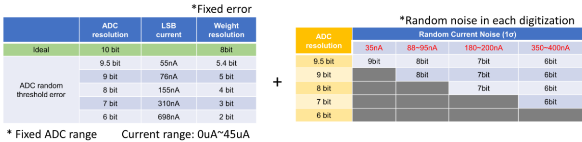
Figure 5-12: Weight mapping. ADC resolution drop can be critical due to fixed error and random noise term.
