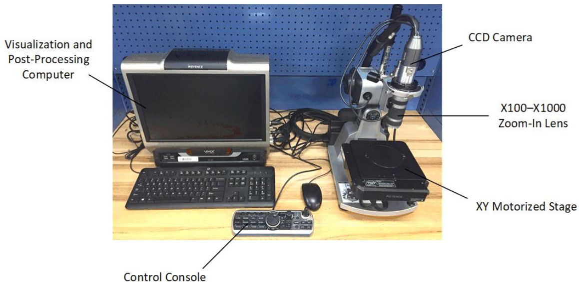
Figure 4.2: VHX-2000 digital microscope and its components
