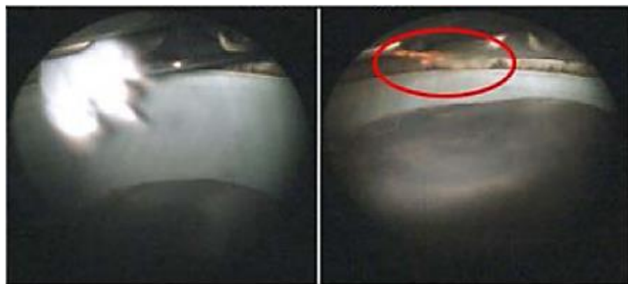
Figure 2.5: An endoscopic image showing a diffusion flame taking place on the injector tip due to the fuel injection process [29]
