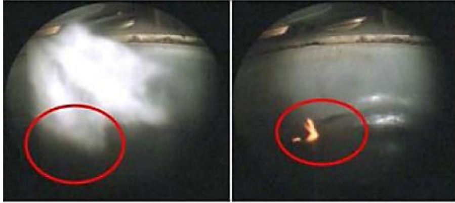
Figure 2.4: An endoscopic image showing a diffusion flame taking place as a result of fuel impingement on the piston's surface during the fuel injection process [29]
