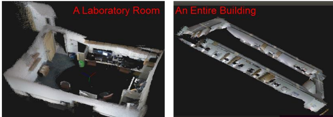
Figure 2.15 Point cloud maps of two environments created based on the proposed system
