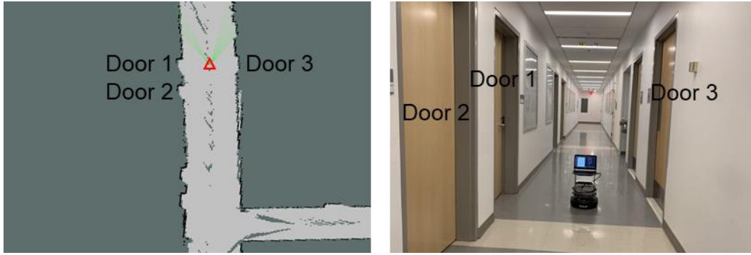
Figure 2.14 Geo-tagged environmental data collection with a TurtleBot platform
