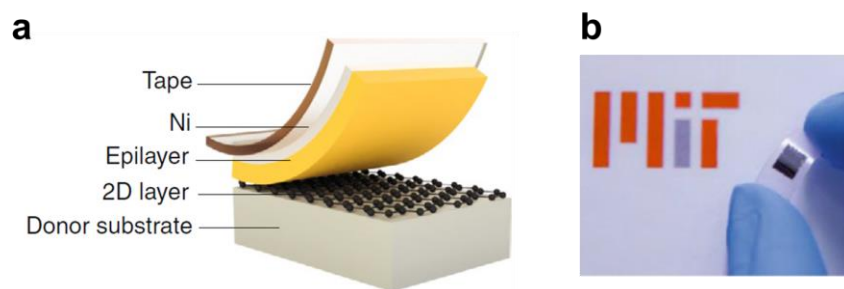
Figure 2.5: Illustration of 2D assisted lift-off process.
