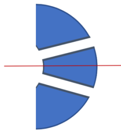
Figure 2.2. Schematic of the nozzle orifice configuration of injector B and C.
