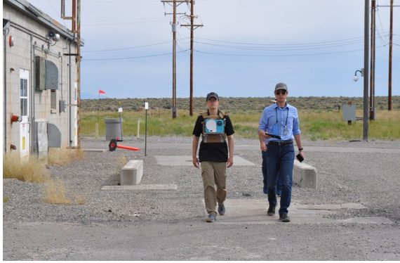
Figure 7.3: Still image of the field experiment conducted at the Idaho National Laboratory. The detector can be seen mounted on the user via the use of a vest and the IMU placed in the foot ware.
