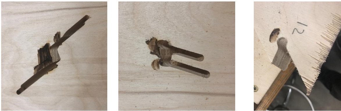
Figure 162_ Collision of the drill collet with material.
