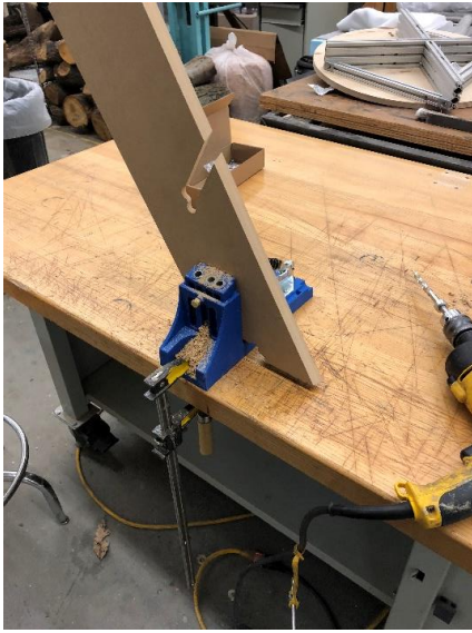
Figure 134_ Application of Kreg jig to drill the connection holes.
