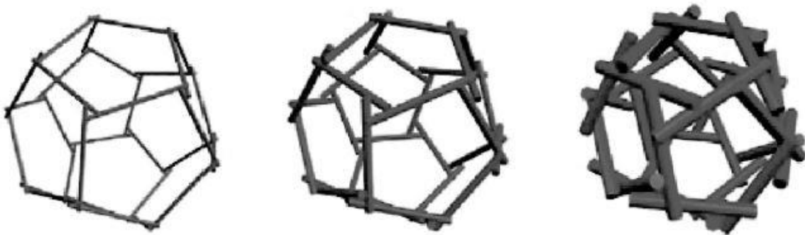
Figure 38_ Reciprocal polyhedra generated by expanding the vertices. Variation in a dodeca-icosahedron for rotation angles 5, 10, and 20 degrees (Sénéchal et al., 2011).
