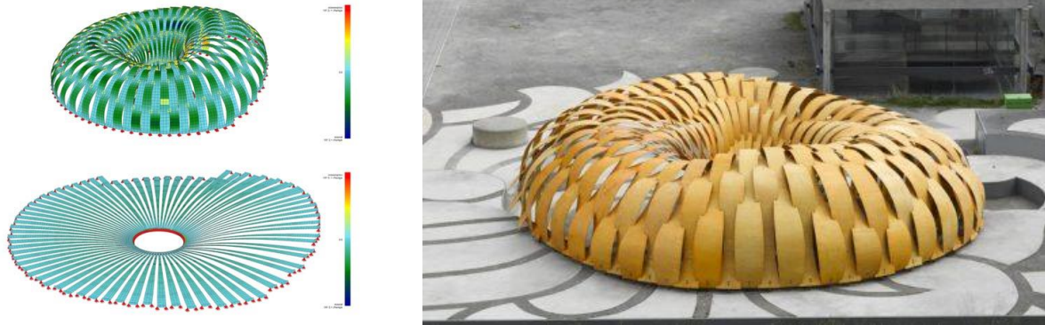
Figure 18_ICD/ITKE Research Pavilion 2010 and application of bending active simulation using FEM to find the global geometry of the interconnected system based on the material behavior under large deformations with predefined connection points (Fleischmann and Menges, 2011).
