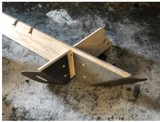
Figure 228_ Connection detailing of the support members and the base plates.
