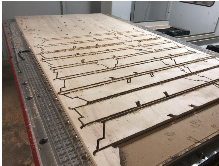
Figure 159_ 5-axis CNC bed and the test cut results for the fabrication test one.
