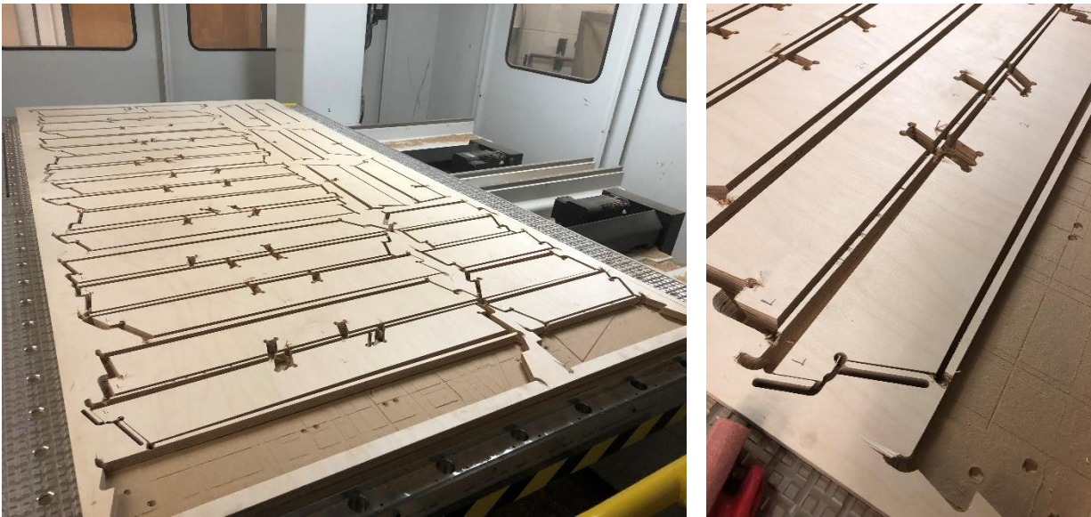
Figure 167_ 5-axis CNC bed and the test cut results for the fabrication test three.
