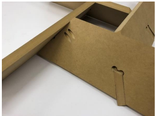
Figure 135_ Modified connection detailing for rotated flat members with Kreg screws.
