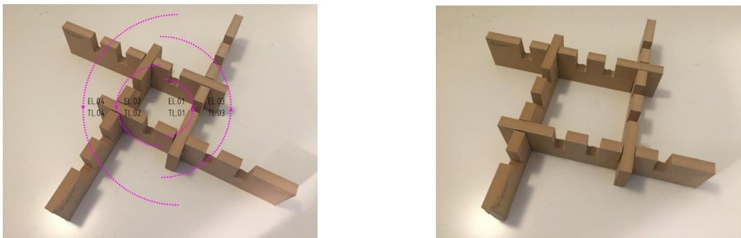
Figure 129_ Conventional reciprocal connection for orthogonal flat members with four different engagement lengths (EL) with different fabrication tolerances (TL).
