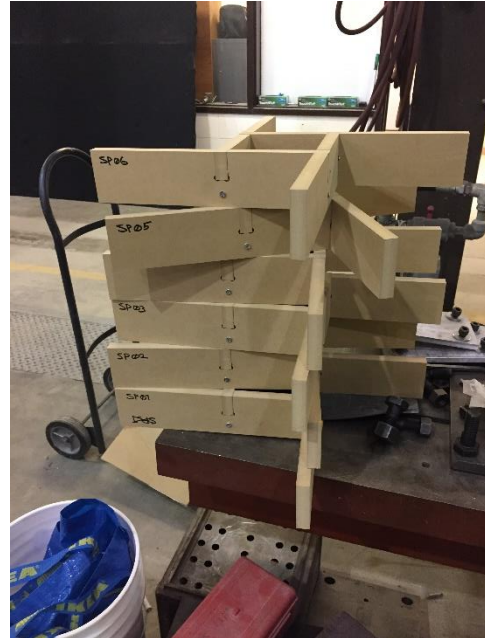
Figure 137_ reciprocal modules are fabricated for structural testing using 3-Axis CNC machine.
