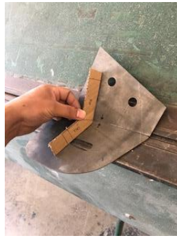
Figure 227_ Bending the supports plates to custom angles using break.
