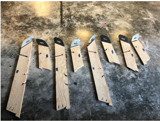
Figure 228_ Connection detailing of the support members and the base plates.
