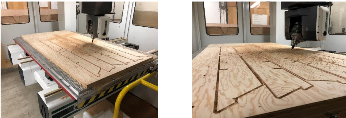
Figure 220_ Cutting the reciprocal members out of plywood sheets using 5-Axis CNC.
