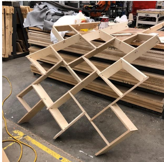
Figure 172_ Bottom up assembly process for the scaled half arch.
