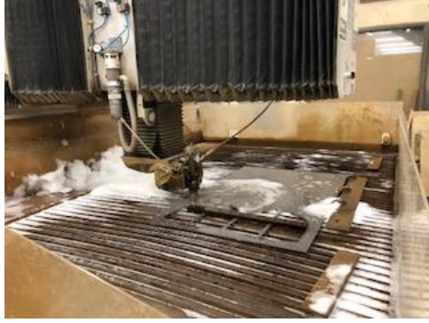
Figure 226_ Fabrication of the support plates using water jet cutter.
