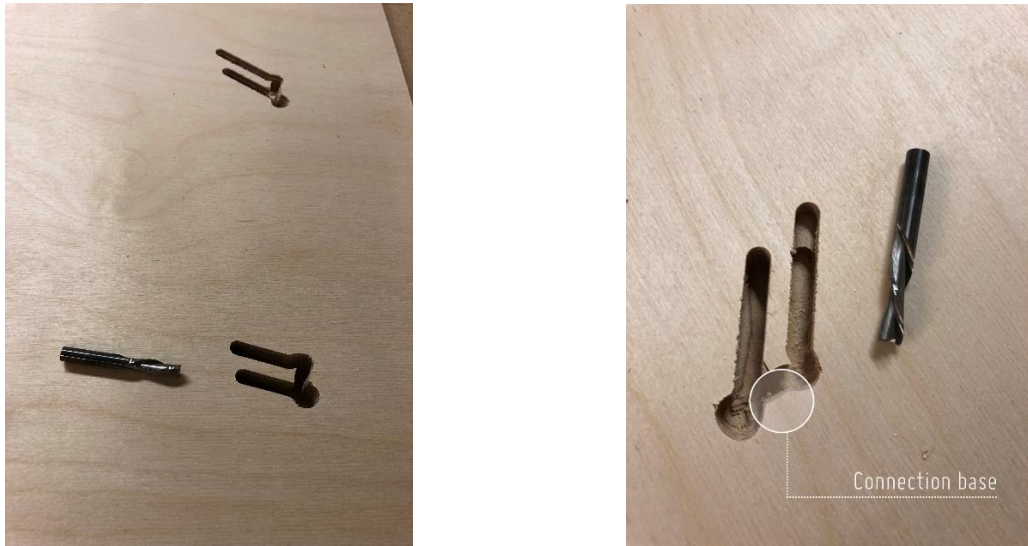
Figure 166_ Drill bit failure in swarf cuts in test two.
