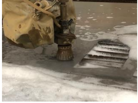
Figure 226_ Fabrication of the support plates using water jet cutter.
