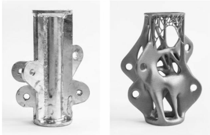
Figure 128_ Topology optimization of metal connection for optimal distribution of material and weight reduction (Galjaard et al., 2014).
