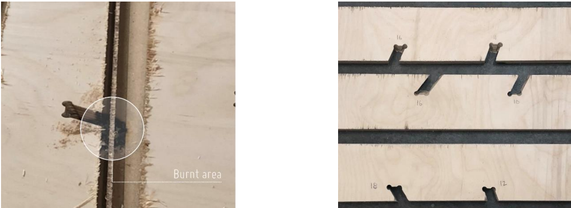
Figure 161_ Excess heat in swarf cuts: Left, burning in the spoil board. right, successful cuts.
