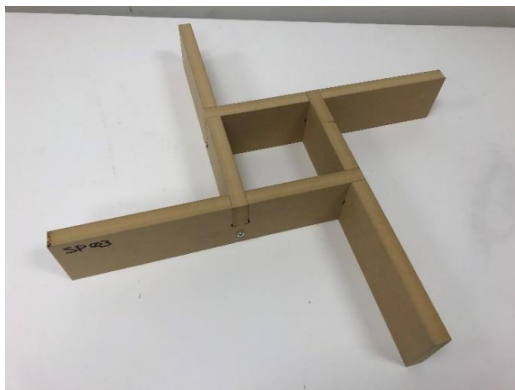
Figure 136_ Modified connection detailing for orthogonal flat members with end grain screw fasteners.
