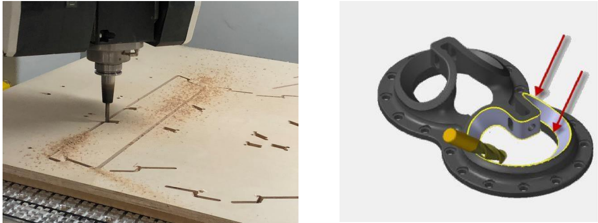
Figure 168_ Using swarf cuts to test the full member cutting in one toolpath.
