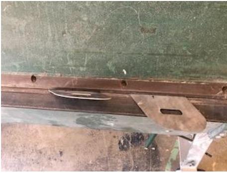
Figure 227_ Bending the supports plates to custom angles using break.
