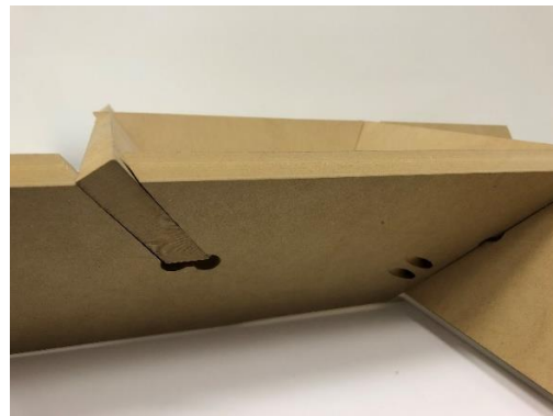
Figure 135_ Modified connection detailing for rotated flat members with Kreg screws.
