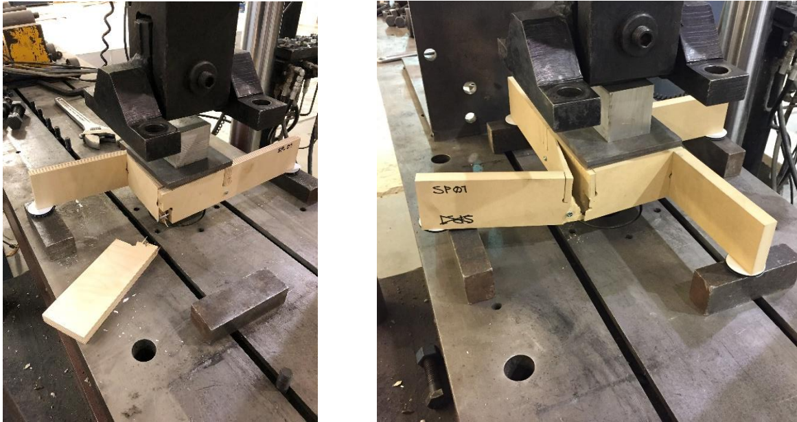
Figure 140_ Failure of test samples under displacement control loading. Left: 13-layer Birch plywood material, right: MDF material.
