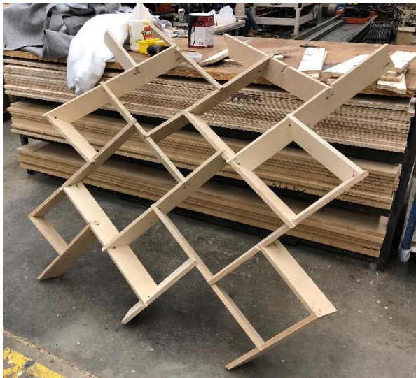
Figure 172_ Bottom up assembly process for the scaled half arch.
