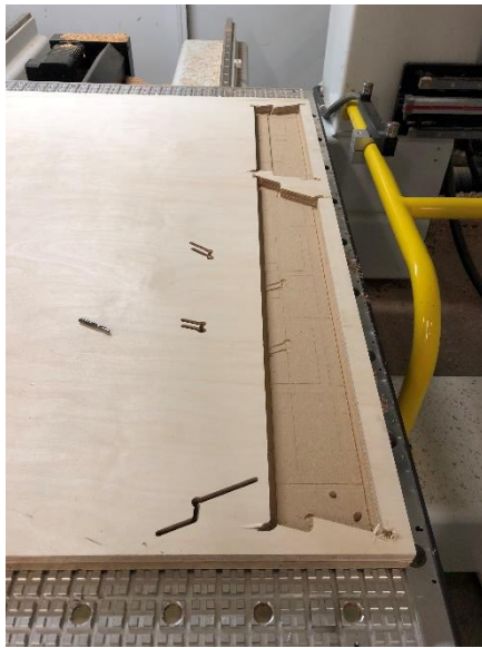
Figure 164_ 5-axis CNC bed and the test cut results for the fabrication test two.
