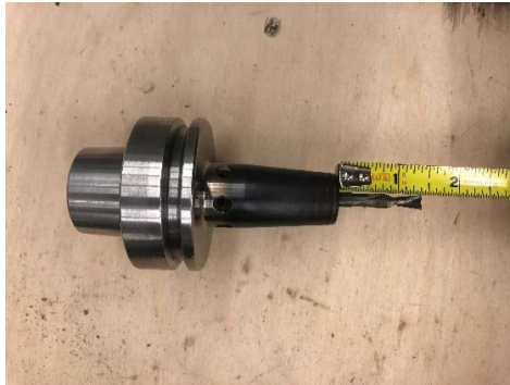
Figure 163_ 1/4 inch down shear drill bit extension capacity.
