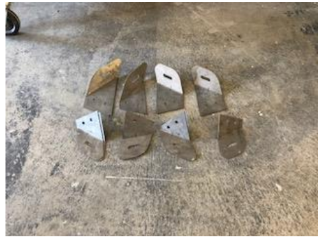
Figure 227_ Bending the supports plates to custom angles using break.
