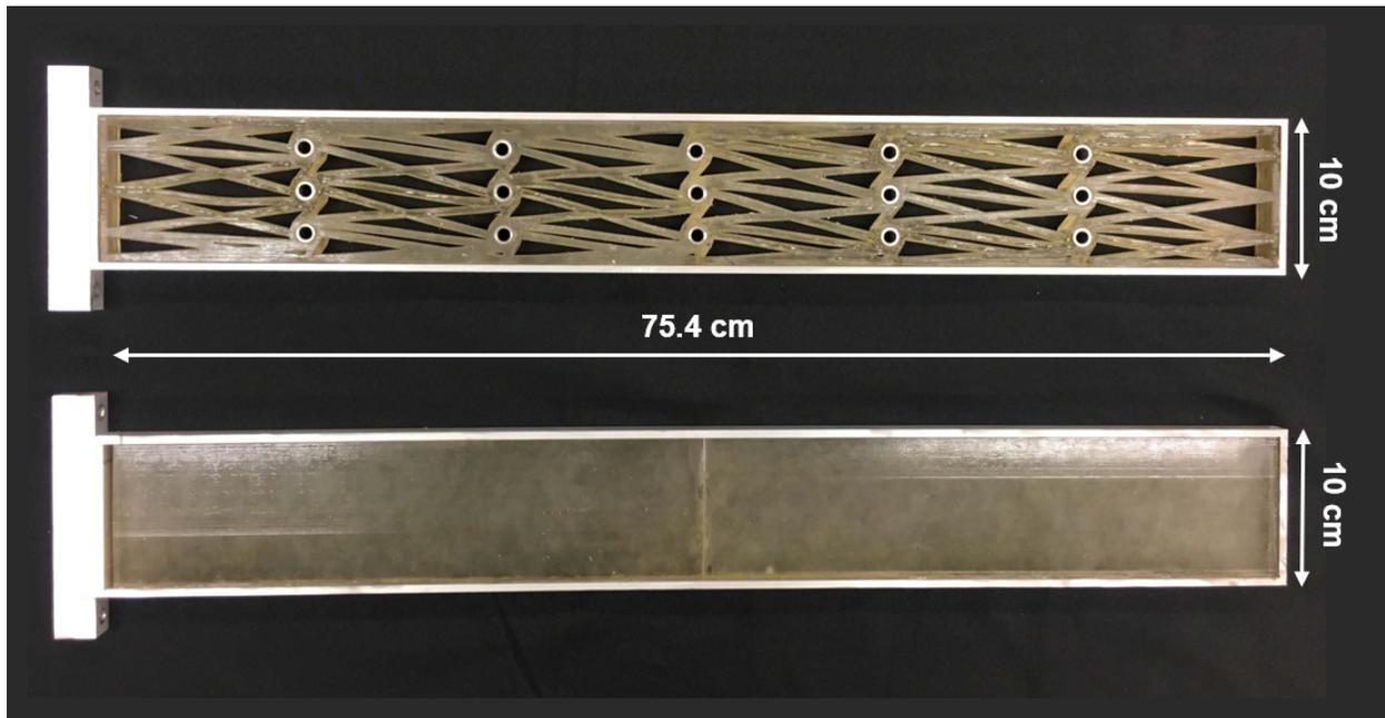
Figure 3.1: Periodic chiral lattice (top) and solid structure (bottom)
