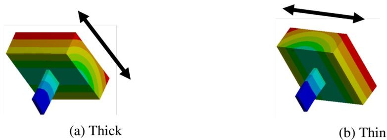
Figure 2.12: Absorber bending direction. Contours show a qualitative absorber displacement.
