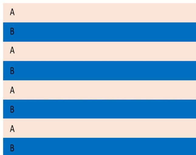
Figure 2.1 Schematic showing structure of a MNL. A and B represent two different metals.
